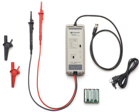
Figure 4. Keysight N2791A 25 MHz differential active probe.
