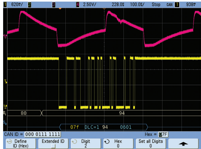
Figure 8. Mixed-signal measurements in a mix-signal automotive system using an MSO
