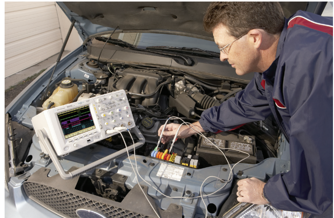
Figure 9. Making remote CAN and LIN measurements with Keysight's battery option for InfiniiVision Series scopes.
