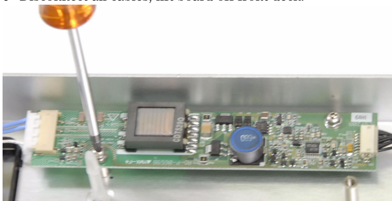
Figure 24 Removal of inverter board
