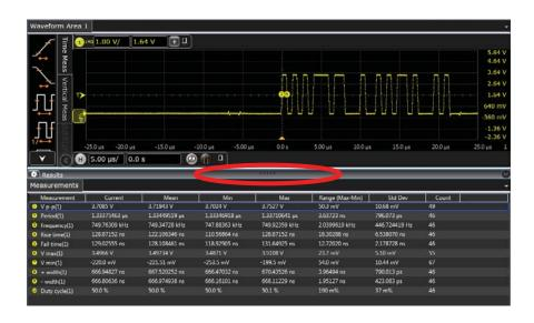
**13** Delete all measurements by right-clicking in the measurement results window and choosing **Delete All Measurements**.
