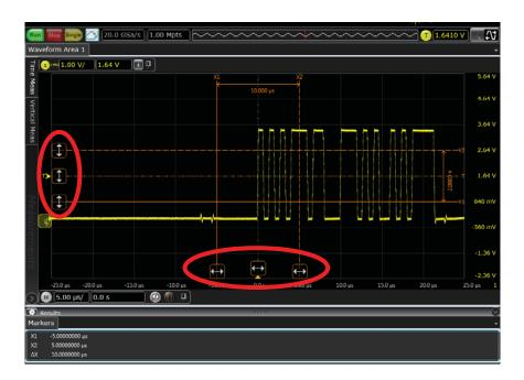
This new Infiniium interface was designed for touch. If you ever tried to move markers with your finger, you know how hard it can be. These handles enable you to easily grab a marker and move it. Experiment now with moving a marker by using a handle.
