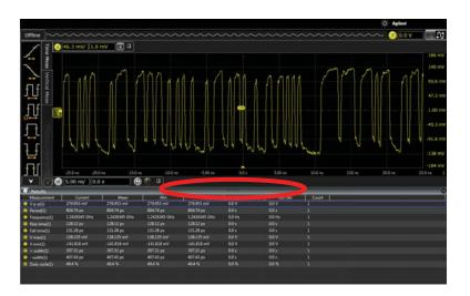
**15** Delete all measurements by right-clicking in the measurement results window and choosing **Delete All Measurements**.
