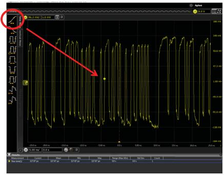
11 To enable measurement callouts, choose **Display > Callouts > Show Measurement**Callouts from the main menu. You will see a measurement callout pinned to the measurement point and can drag the callout to any location on the display. This capability is very useful for documentation because a single screen shot can now show the measurement data right on the screen.
