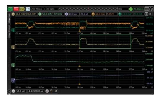
23 To determine how much energy is consumed over 1 cycle, drag and drop the Vmax measurement onto f3 to show how many joules are consumed in a single pulse.
