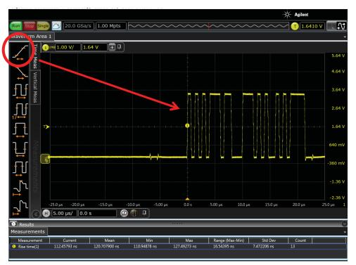
9 To enable measurement callouts, choose **Display > Callouts > Show Measurement**Callouts from the main menu. You will see a measurement callout pinned to the measurement point and can drag the callout to any location on the display. This capability is very useful for documentation because a single screen shot can now show the measurement data right on the screen.
