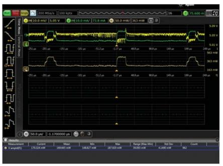
14 Click the **Vertical Meas** tab on the left side of the display, then drag-and-drop the **Vmax** and **Vmin** measurements onto **f1** so you can see maximum and minimum power values.
