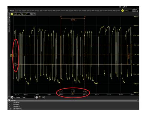
**8** Turn the markers off by clicking the Markers button again and then setting the **Mode** to **Off** in the Markers Setup dialog box.
