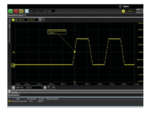
23 Experiment with moving these bookmarks to anywhere on the screen. You can also move the anchor point to different locations on the waveform. This capability is useful for collaboration between multiple people, as you can create bookmarks, save the setup as a composite file (.osc), and send that file to a colleague. When that person opens the file on their oscilloscope or laptop, they will be able to navigate through the waveform and see all of the bookmarks.
