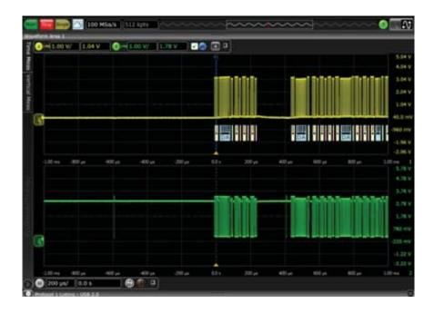
A better way is to use segmented memory to capture all Setup packets.
