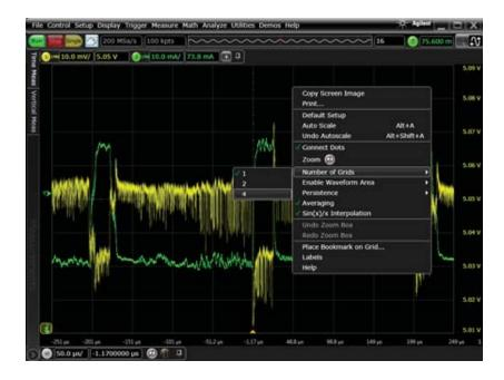
11 Turn on Function 1 (Math > Functions...) and make it equal to channel 1 \* channel 2 (V\*l) as shown below.
