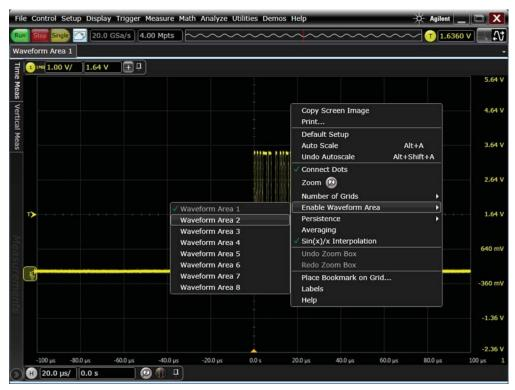
**4** Experiment with the new waveform area, such as by moving a waveform from one area to another. Using the custom tabbed view, you can even drag waveform areas to another monitor.
