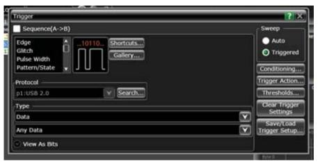
**11** Move the mouse to generate USB data packets that contain XY coordinates. The scope now triggers only when data packets are transmitted.
