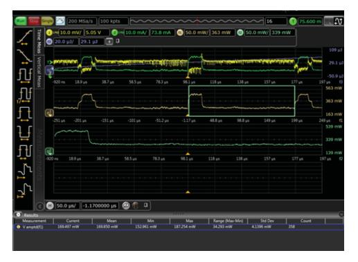
Now that function 2 has been set up to create a gate for a single cycle, you can use this gate to determine power consumption over one cycle.
