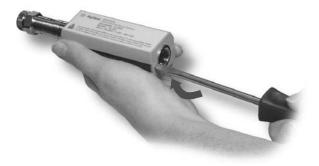
Figure 12 Removing Power Sensor Shell
