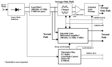
Figure 1 Simplified Sensor Block Diagram
