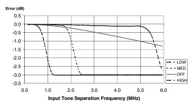
Figure 9 Filter responses for the E9323A and E9327A power sensors (High, Medium, Low, and Off)
