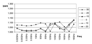
Figure 2 TypicI SWR (50 MHz to 18 GHz) for the E9321A and E9325A sensors at various power levels
