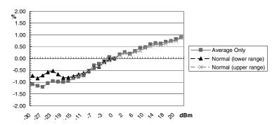
Figure 5 Typical Power Linearity at 25°C for E9323A and E9327A
