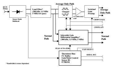
Figure 11 Simplified Sensor Block Diagram
