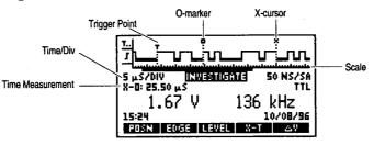
• Use three steps to measure time. First, move the X-cursor to a point of interest using (and b). Then, move the O-marker to the X-cursor position with (a). Finally, move the X-cursor to the next point of interest and read the time in the display.
