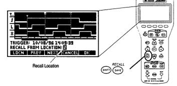
• There are 10 waveform storage locations, numbered from 1 to 10. Press **NEXT** or **NEXT** to select a storage location. When the desired location is selected, press **NOXT** to recall the waveform and setup.
