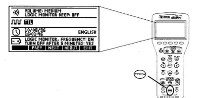
To use System Setup, move the highlight (white text on a black background) to the area of interest and then change the values for that setting. The Logic Family setting, TTL, is highlighted in the screen above.
