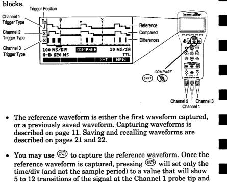
• To erase the reference waveform, press NER. You can then capture a new reference waveform.
