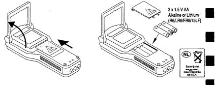
HP LogicDart calibration is not affected by dead batteries or the battery replacement procedure.
