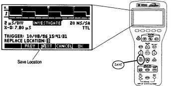
• There are 10 waveform storage locations, numbered from 1 to 10. Press NET or PREV to select a storage location. When the desired location is selected, press to save the waveform and setup.
