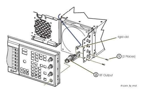
Figure 3-50 RF Output Connector for Option 1EM
