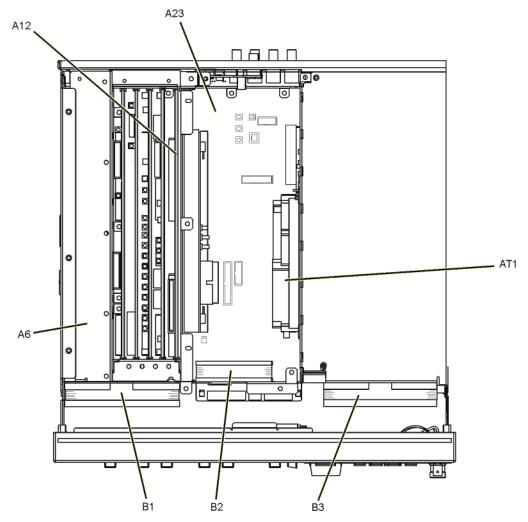
Figure 2-3 E4438C Assemblies from a Top View (Option 501, 502, 503, 504 or Option 300)
