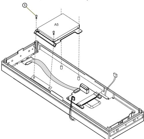
Figure 3-17 A5 Hard Drive, for instruments with serial prefix ≥ US4426/MY4426
