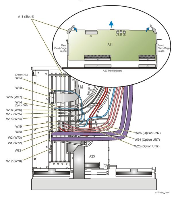
Figure 3-22 All Internal Bit Error Rate Analyzer
