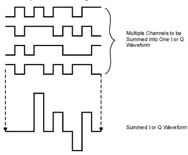
The I and Q waveforms combine in the I/Q modulator to create an RF waveform. The magnitude of the RF envelope is determined by the equation  $\sqrt{I^2+Q^2}$ , where the squaring of I and Q always results in a positive value.
