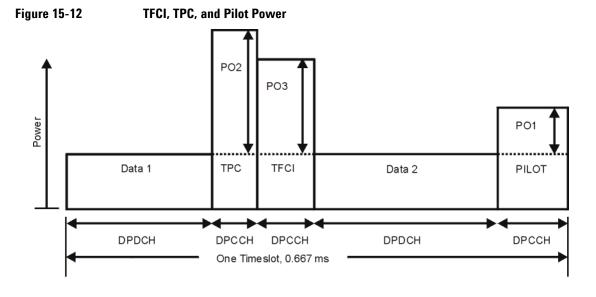
The display in Figure 15-13 shows that the channel in row 6 of the table editor has the data transmit power (Power dB) set to -6.02 dB with the following offsets: TFCI Power set to 2.00 dB, TPC Power set to 3.00 dB, and Pilot Power set to 1.00 dB. Because of these offsets, the control symbols corresponding to TFCI, TPC, and Pilot will transmit at -4.02 dB, -3.02 dB, and -5.02 dB respectively.
