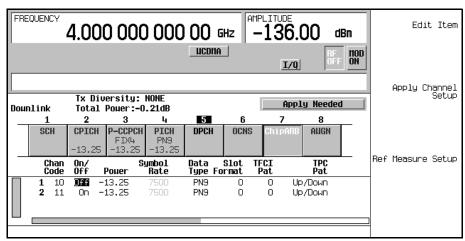
Figure 17-6 Display Indicates that Apply is Needed
