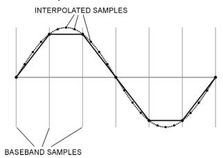
The interpolation filters in the DACs have overshoot. If a baseband waveform has a fast-rising edge, the interpolator filter's overshoot or frequency response becomes a component of the interpolated baseband waveform. This response causes a ripple or ringing effect at the peak of the rising edge. If this ripple exceeds (or overshoots) the upper limit of the DAC's range, the interpolator calculates erroneous sample points and
