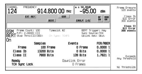
6. Press the **Trigger** hardkey to start the measurement:
