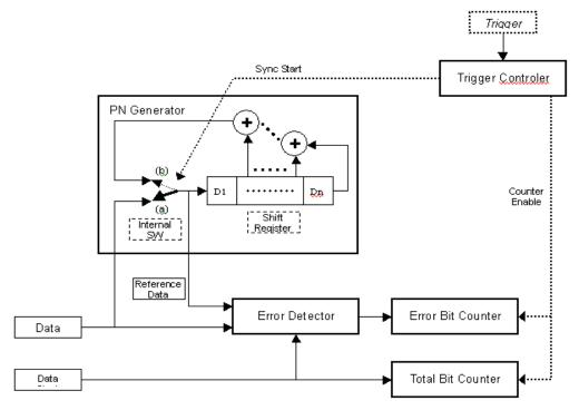
In this example, the triggering sequence is where you have an incoming data clock and data bit sequences, the trigger is active, and the BERT measurement begins. Refer to Figure 9-25.
