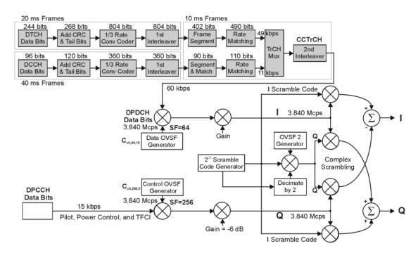
NOTE: Shaded areas of the graphic indicate pre-calculated values based on the user's collection of data and coding parameters. Multiplexing and spreading are done real time.
