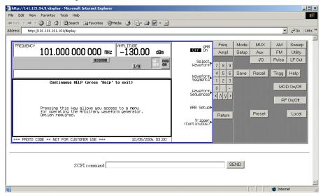
This web page remotely accesses all signal generator functions and operations. Use the mouse pointer to click on the signal generator's hardkeys and softkeys. The results of each mouse click selection will be displayed on the web page. For example, click on the Frequency hardkey then use the front panel key pad to enter a frequency. You can also use the up and down arrow keys to increase or decrease the frequency.
