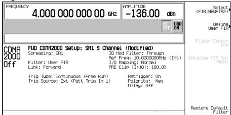
The filter you selected is NEWFIR2. You can see the name displayed below the **Select** softkey. In the Filter field, near the left of the display, User FIR is displayed to indicate that a user-defined FIR filter has been selected.
