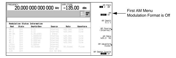
Active Modulation Format Annunciator 20.000 000 000 000 6Hz -135.00 dBm First AM Menu Off On Modulation format is On Modulation Status Information flod State Depth/Dev Source Rate **Haveform** AM Source (Internal) AN 1 0n 0.1% Internal 400.OHz Sine AM Rate 400.0 Hz AM Waveform (Sine) Internal Internal Ext1 DC Ext 50 Ohm AM Depth Couple
