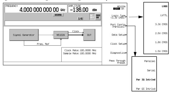
1. Refer to Figure 7-10. Press the **Logic Type** softkey. From this menu, choose a logic type.
