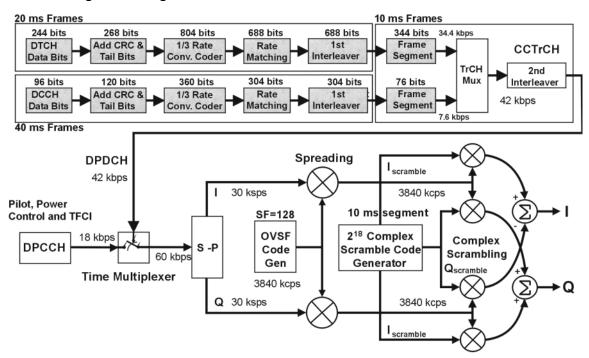
NOTE: Shaded areas of the graphic indicate pre-calculated values based on the user's collection of data and coding parameters. Multiplexing, scrambling and spreading are done real-time.
