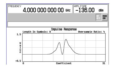
Refer to Figure 4-33 on page 174. The graphic display can provide a useful troubleshooting tool (in this case, it indicates that a coefficient value is missing, resulting in an improper Gaussian response).
