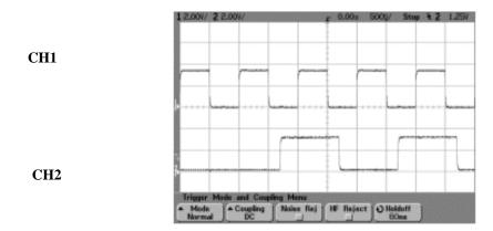
CH1: BER TEST OUT (pin 20 of AUX I/O connector) CH2: BER MEAS END (pin 1 of AUX I/O connector)
