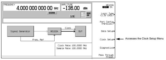
From this softkey menu, set all of the clock parameters that synchronize the clocks between the N5102A module and the ESG. You can also change the clock signal phase so the clock occurs during the valid portion of the data. Figure 7-14 shows the clock setup menu.
