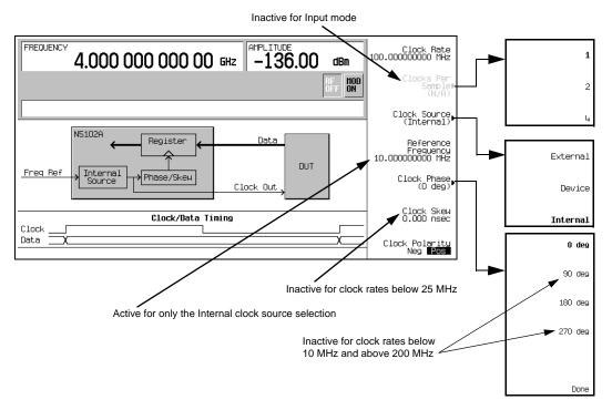
The top graphic on the display shows the current clock source that provides the output clock signal at the Clock Out and Device Interface connectors. The graphic changes to reflect the clock source selection discussed later in this procedure. The bottom graphic shows the clock edges relative to the data. The displayed clock signal will change to reflect the following:
