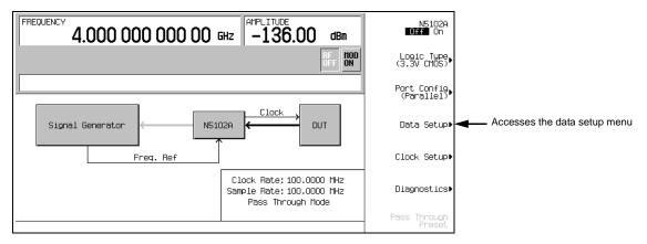
This softkey menu accesses the various parameters that govern the data received by the ESG The status area of the display shows the number of data lines used for both I and Q along with the clock position relative to the data. Figure 7-20 shows the data setup menu structure.
