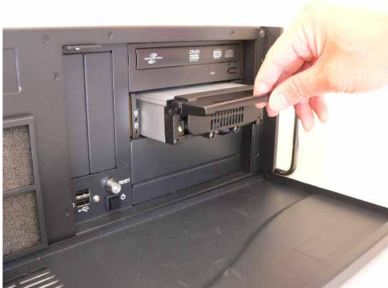
Figure 39 Ejector Lever Pulled Up
