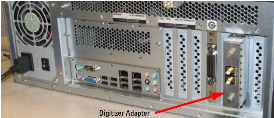
Figure 3 Connect adapter to back of PC digitizer card
