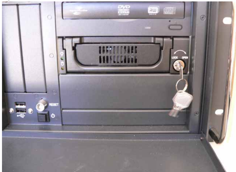
Figure 38 Hard Disk Drive Assembly
