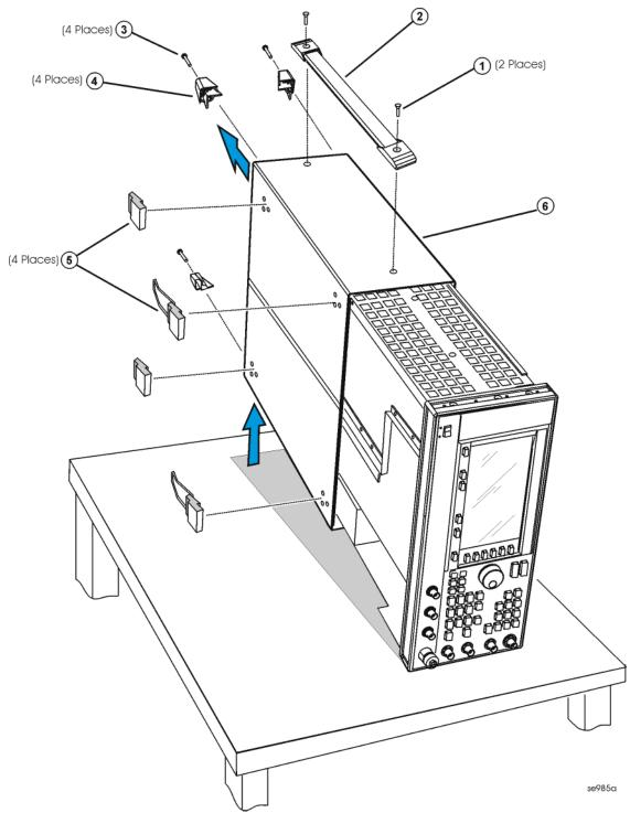
Figure 4 Inner Top Cover Removal
