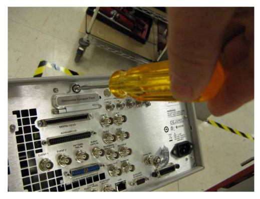
2. Install the IC flash memory card provided with the upgrade kit.
