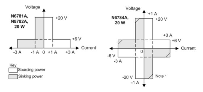
Note 1. When sinking power, the N6784A model can operate at the maximum rated output power for only a limited amount of time. The unit monitors the temperature of the internal power devices and latches the output off if the output power has exceeded its safe limits. A protect clear is required to resume normal operation. The condition is annunciated by the OT status bit. Refer to the downprogrammer derating figure for the values of the safe limit boundaries.
