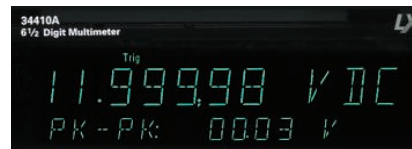
Figure 3. An example of a DMM that can display both DC and AC voltage measurements simultaneously (34410A/11A DMMs)
