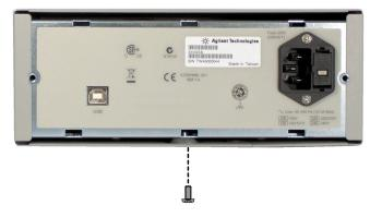
**5 Remove the cover**. Remove the screw in the bottom of the cover and slide the cover off the instrument.
