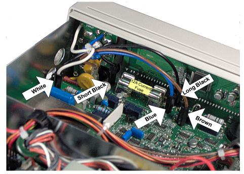
9 Disconnect the individual front panel wires shown below.
