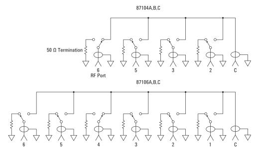
Figure 1. Keysight 87104A/B/C and 87106A/B/C simplified schematics
