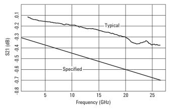
Figure 7. Insertion loss
