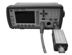
5 Connect the sensor to the POWER REF connector.
