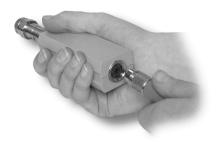
2 Connect the other end of the 11730A cable to the CHANNEL A (or CHANNEL B) input connector.
