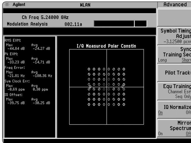
Figure 4. Constellation of 54 Mbps OFDM signal showing overlaid 64QAM and BPSK points.
