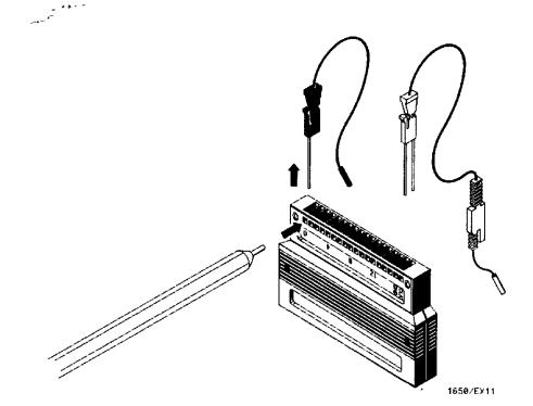
You re-connect a probe to a pod by inserting the double pin end of the probe into the pod. The probes and pod connector body are both keyed (chamfered) so that they will fit together in only one way.
