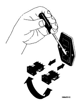
You change the line voltage setting by pulling the fuse module out and reinserting it with the proper arrows aligned. To remove the fuse module, carefully pry at the top center of the module (as shown) until you can grasp it and pull it out by hand.
