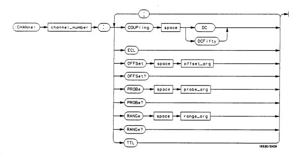
**channel\_number** = An integer from 1 through 8, depending on how many acquisition cards are installed in the oscilloscope
