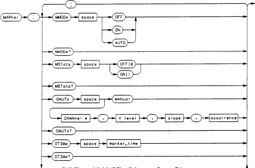
P/O Figure 6-1. MARKer Subsystem Syntax Diagram
