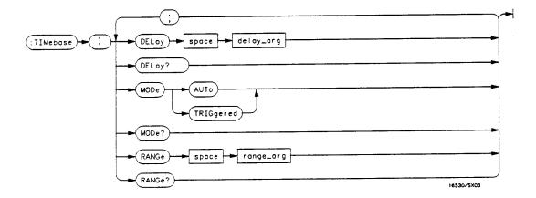
delay\_arg = delay time in seconds, from -2500 seconds through +2500 seconds range\_arg = a real number from 5ns through 10s
