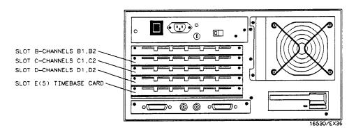
Figure 5-2. Oscilloscope Label Identification.
