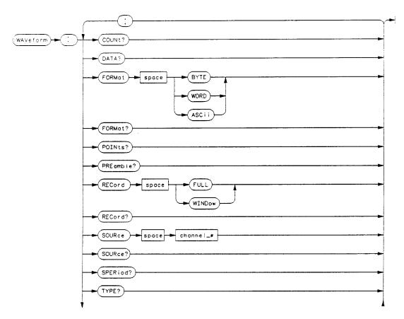
P/O Figure 10-3. WAVeform Subsystem Syntax Diagram
