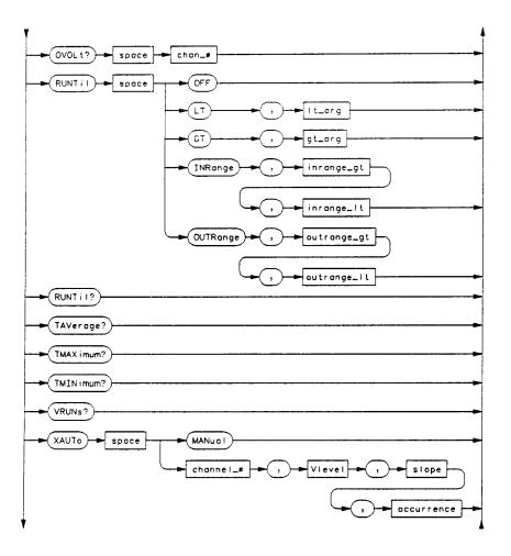
P/O Figure 6-1. MARKer Subsystem Syntax Diagram
