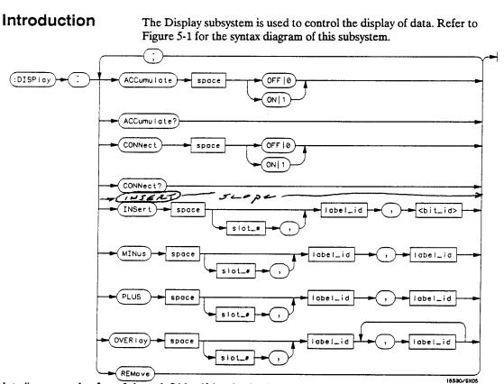
$slot_{\#} = a$  number from 1 through 5 identifying the timebase card slot
