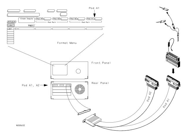
**Connecting Probe Cables to the Logic Analyzer**
