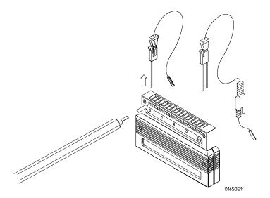
**Installing Probe Leads**
