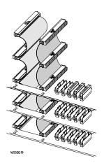
6 Feed the free end of the 2x10 cables of the expander cards through the access holes to the master card. Plug the 2x10 cables into J4 (bottom-most expander in a five-card configuration) and J5 (expander that is next to the master card) on the master card.
