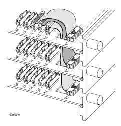
7 Place the remaining expander boards on top of the master board. Feed the 2x25 cables that are plugged into the master card through the cable access holes of the expander cards. Plug the 2x25 cables into J9 and J10 of the expander cards.
