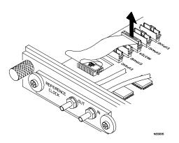
5 Place the master card on top of any expander cards that are under the master card. Feed the 2x25 cables that are plugged into the master card through the cable access holes of the expander cards. Plug the 2x25 cables into J9 and J10 of the expander cards.
