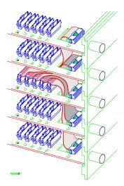
9 The following illustration shows the proper connection of the 2x25 cables and the 2x10 cables for a five card module. If a two-, three-, or four-card module was configured, not all cables will be present; however, the existing cables will be routed in the same manner. Make sure ALL cables are firmly seated.
