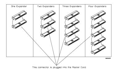
3 Look at the illustration in the previous step. The illustration shows which of the cable connectors is plugged into the master card. Plug one 2x25 cable into the master card J9. Observe which cable connector (as shown in the illustration) is plugged into J9. Follow the same procedure to connect the second 2x25 cable into the master card J10.
