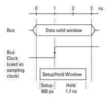
(The actual sampling position is in the middle of the setup/hold window.)
