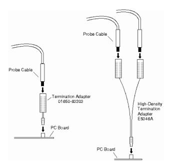
Both the 01650-63203 and the E5346A adapters include termination for the logic analyzer. The 01650-63203 termination adapter plugs into a 2 x 10 pin header with 0.1 inch spacing. The E5346A high-density adapter connects to an AMP "Mictor 38" connector. If possible, use support shrouds around the Mictor connector to relieve strain and improve connections.
