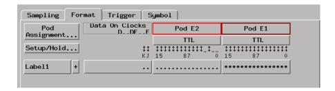
The Format tab lets you assign bus and signal names (from the device under test), to logic analyzer channels. These names are called *labels*. Labels are used when setting up triggers and displaying captured data.
