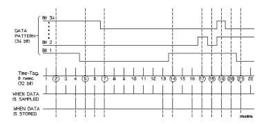
In most cases a transitional timing trace is stored by a mixture of the minimum and maximum cases. Therefore, in this example the actual number of transitions stored will be between 1023 and 2047.
