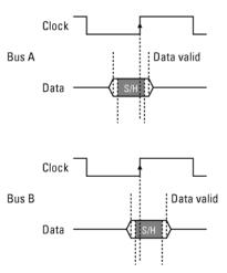
To position the setup/hold window (sampling position) within the data valid window, a logic analyzer has an adjustable delay on each sampling clock input (to position the setup/hold window for all the channels in a pod).
