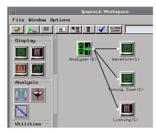
3. Drag the display tool icon and drop it on the analyzer icon.
