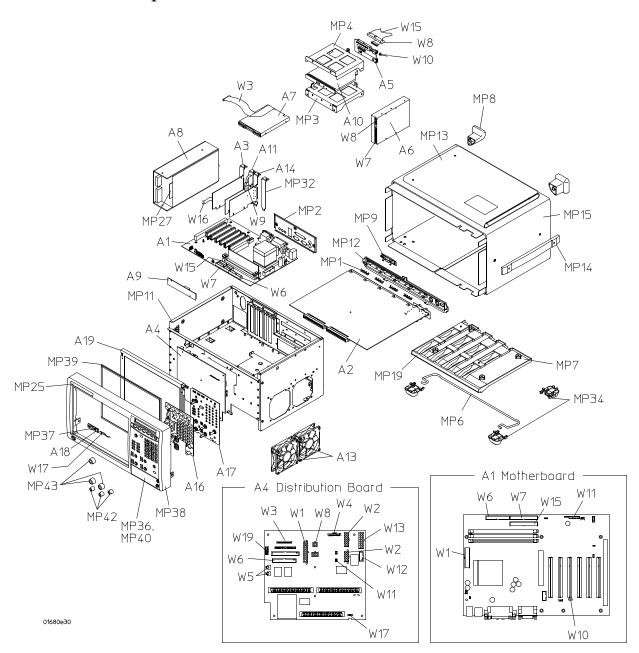
Exploded view of the Agilent 1680A,AD-series logic analyzer
