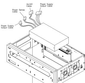
**5** Lift the power supply out of the chassis.
