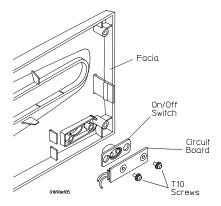
Reverse this procedure to assemble the fascia.
