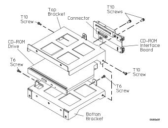
**5** Reverse this procedure to reassemble and install the CD-ROM drive. Ensure the motherboard is properly installed before installing the CD-ROM drive.
