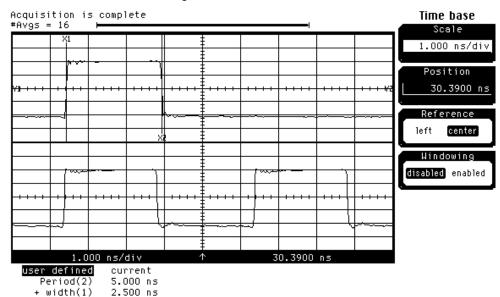
**c** If the pulse width is outside the limits, adjust the pulse generator channel 2 width until the pulse width is within limits.
