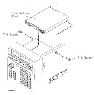
When installing a new flexible disk drive, industrial double-sided tape (Agilent 0460-2010 or similar) is required to dress the cable onto the flexible disk drive. Apply the tape as shown.
