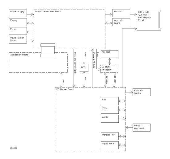
Agilent 1680A, AD-Series Logic Analyzer Block Diagram
