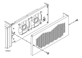
**3** After the required power-on troubleshooting and repair is complete, reverse the above procedure to remove the fan guard and reassemble the instrument.
