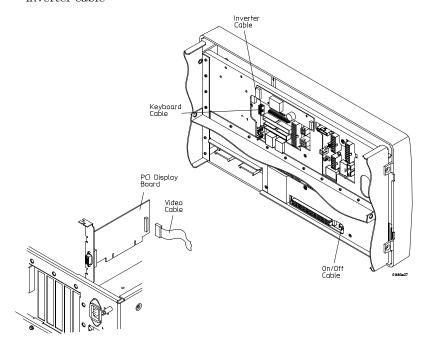
**5** Using a Torx T-15 screwdriver, remove four screws that secure the front panel assembly to the chassis. Lift the front panel assembly away from the chassis.
