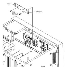
**5** Reverse this procedure to install the inverter board.
