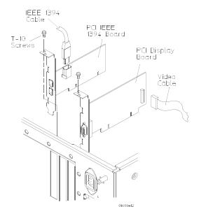
**5** Reverse this procedure to install the PCI boards.
