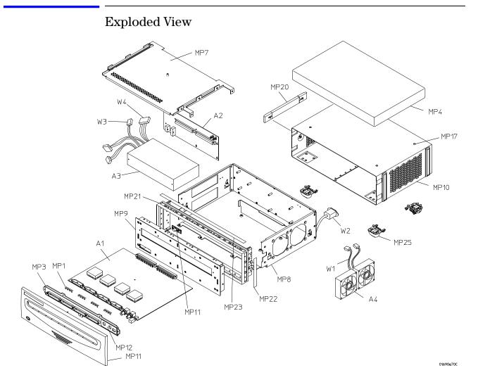
Exploded view of the Agilent 1690A, AD-series logic analyzer
