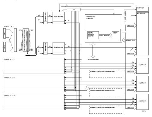
**Probing.** The probing system consists of a tip network, a probe cable, and terminations that reside on the analyzer board. Each probe cable is made up of two ribbonized coaxial cables carrying 16 data channels and 1 clock/data channel.
