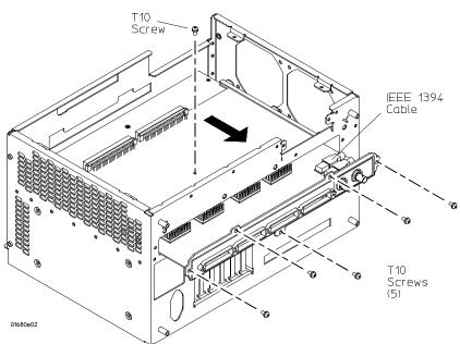
**6** Slide the acquisition board out the rear panel of the logic analyzer.
