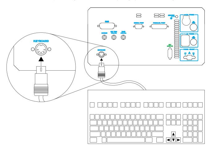
**3** Connect the other end of the keyboard cable to the keyboard.
