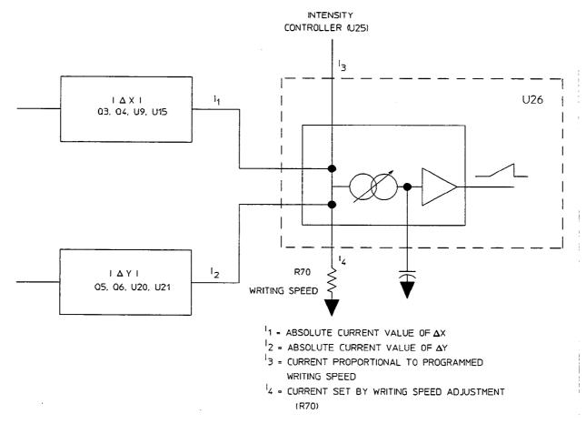
8-3. Ramp Generator Simplified Block Diagram
