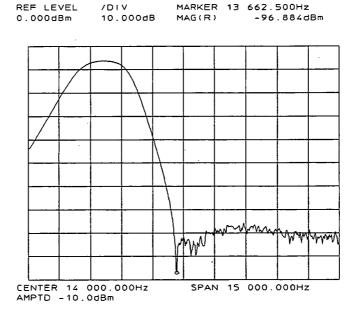
Figure 5-2. 14kHz Filter Response
