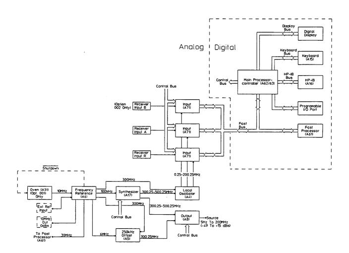
Figure 2-10. HP 3577B Overall Block Diagram
