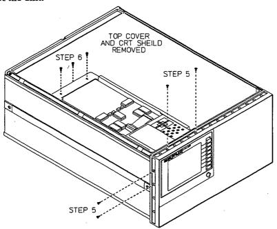
Figure 5-6. Removing the Display
