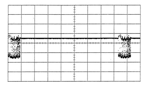
Figure 5-25. Focus A80 TP1 Normal Operation with Centered Focus Pot
