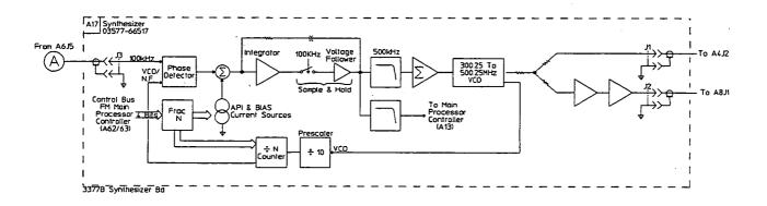
Figure 2-4. HP 3577B Functional Block Diagram (A5/A17) Part 2 of 6
