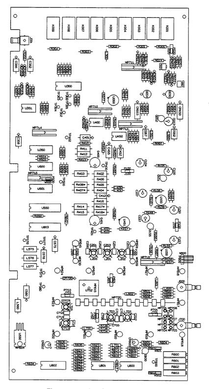
Figure 9-14. A18 Component Locator
