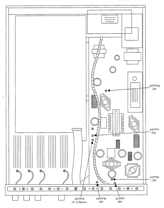
Figure 2-1. Fault Isolation Test Signal Locations
