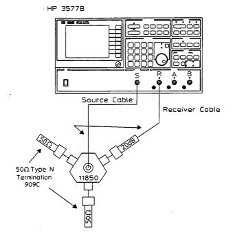
Figure 3-16. Source Flatness and Absolute Accuracy Test Set-Up
