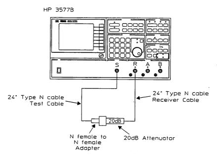
Figure 3-14. Calibration of Transmission Loss from **Power Splitter to Channel R**
