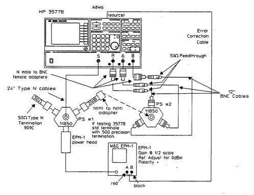
Figure 3-9. Receiver Flatness and Absolute Accuracy Test Set-Up (1  $M\Omega$ )
