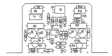
Figure 5-23. A80 Adjustment Locations for Final Focus
