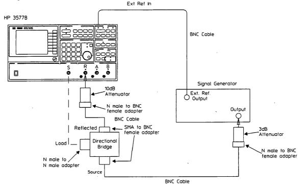
Figure 5-5. On Carrier Return Loss Adjustment Test Set-up
