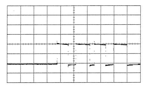
Figure 5-31. Z-Amplifier Auxiliary Output Vertical attenuator =  $500 \,\mu\text{V/Div}$  Sweep =  $100 \,\mu\text{s/Div}$
