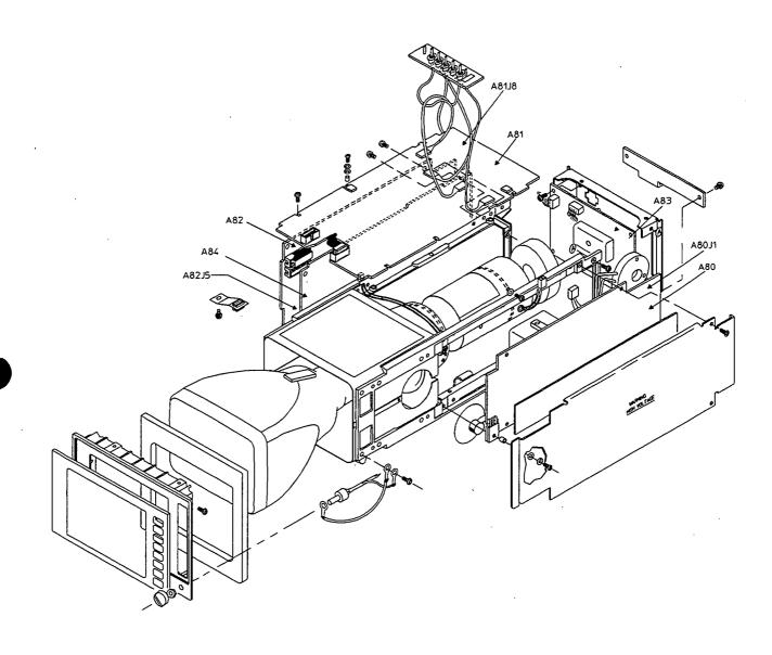
Figure 6-6. HP Digital Display Assembly Locations
