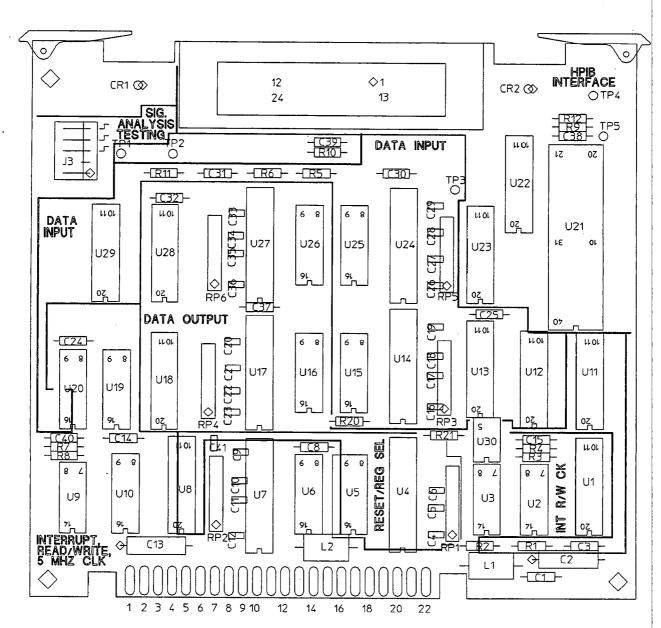
Figure 9-10. A16 Component Locator
