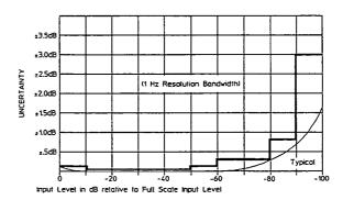
Frequency Response: Specifications apply when inputs are driven from a  $50\Omega$  source impedance.
