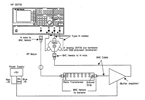
Figure 3-5. Dynamic Linearity Test Set-Up
