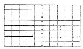
Auxiliary Z Output at A81 J3 .5 V/Div 100  $\mu$  s/Div
