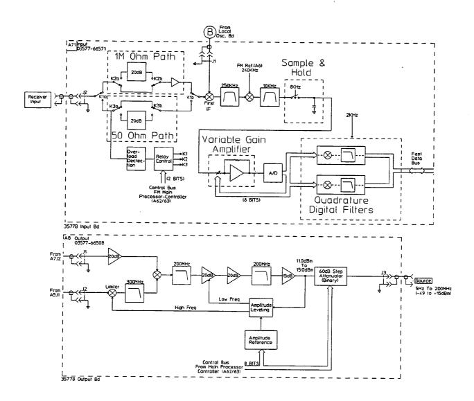
Figure 2-6. HP 3577B Functional Block Diagram, (A71/A8) Part 4 of 6
