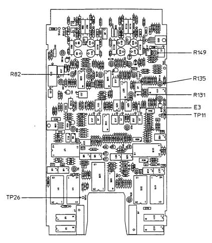
Figure 5-22. A81 Adjustment Locations for Final Focus
