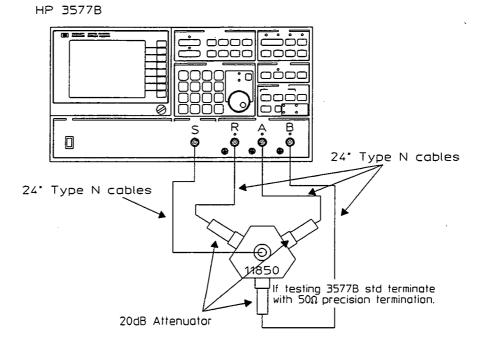
Figure 3-10. Receiver Power Splitter Calibration
