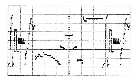
Figure 5-30. Y-Amplifier Auxiliary Output Vertical attenuator = 200 mV/Div Sweep = 2 ms/Div
