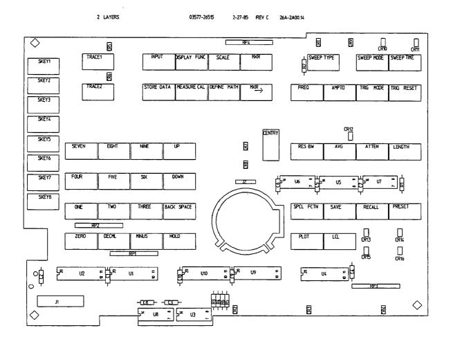
Figure 9-9. A15 Component Locator
