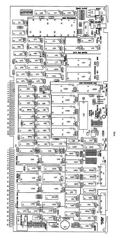
Figure 9-24. A62/63 Component Locator
