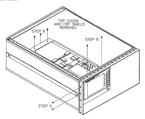
Figure 9-25. Digital Display Removal
