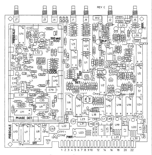
Figure 9-8. A6 Component Locator
