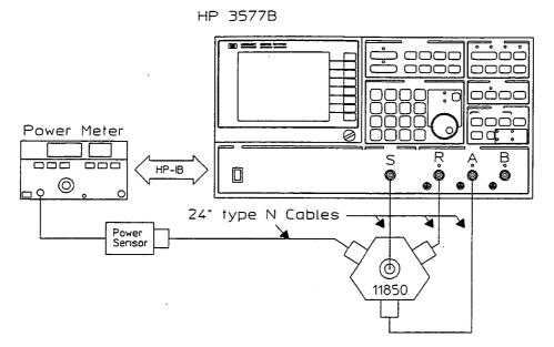
Figure 5-3. Input Level Calibration Test Set-up
