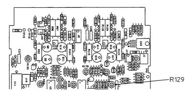
Figure 5-13. A81 Adjustment Locations for High Voltage Power Supply
