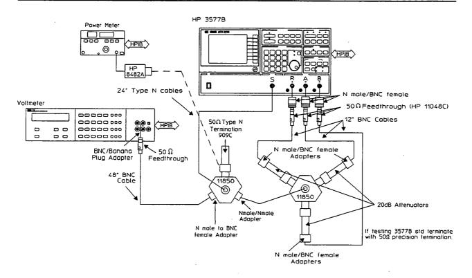
Figure 3-12. Absolute Accuracy and Flatness Test Set-Up ( 1  $M\Omega$  )
