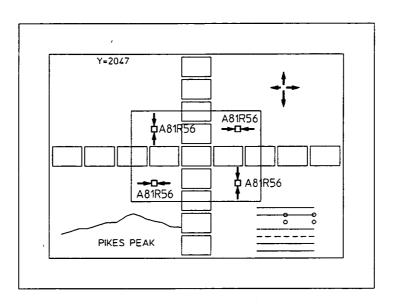
Figure 5-20. Stroke Intensity Adjustment Test Pattern
