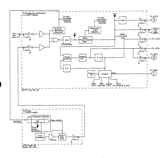
Figure 2-3. HP 3577B Functional Block Diagram (A6/A31) Part 1 of 6
