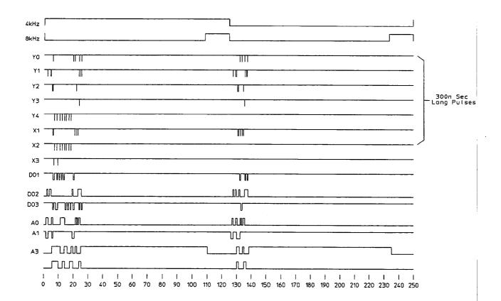
Figure 9-17. A19 Circuit Board Signature Analysis D
