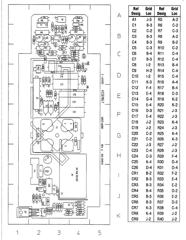
A80 High Voltage Power Supply Component Locator Rev A
