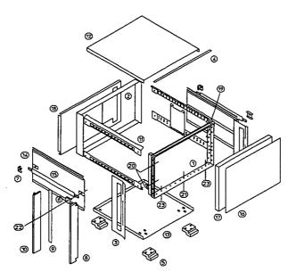
Figure 6-1. Cabinet Parts, Exploded View
