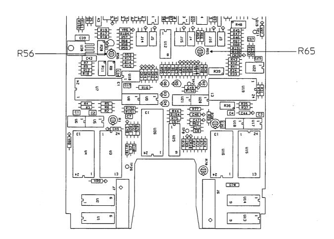
Figure 5-21. A81 Adjustment Locations for Stroke Intensity
