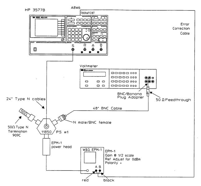
Figure 3-18. EPM-1 Flatness Test Setup
