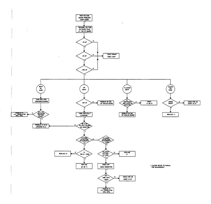
Figure 9-32. A80 High Voltage Power Supply Troubleshooting Procedure
