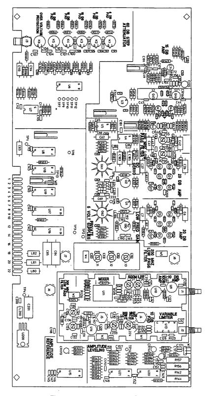
Figure 7-1. A8 Component Locator
