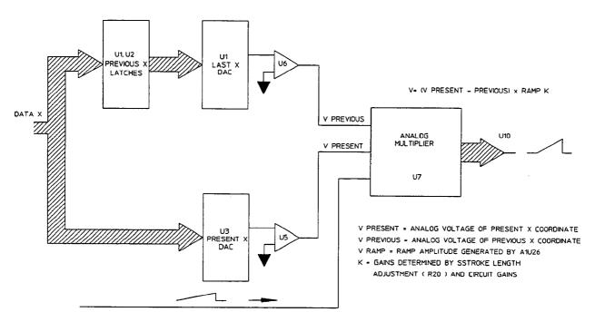
Figure 8-2. Analog Multiplier Simplified Block Diagram
