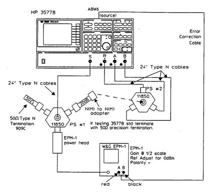
Figure 3-8. Receiver Flatness and Absolute Accuracy Test Set-Up (50  $\Omega$ )
