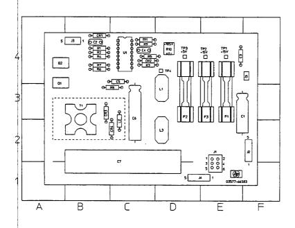
A83 Low Voltage Power Supply Component Locator Rev A
