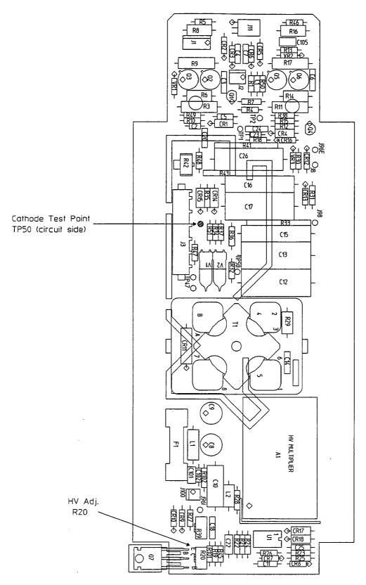
Figure 5-14. A80 Adjustment Locations for High Voltage Power Supply
