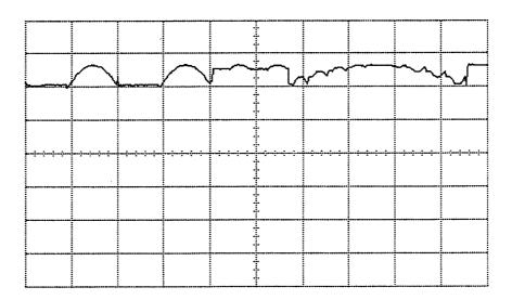
Figure 5-24. XFOC Testpoint 11 Vertical attenuator = 1 V/Div Sweep =  $100 \mu s/Div$
