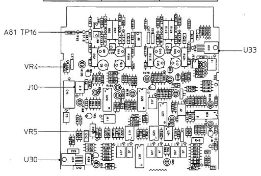
Figure 5-11. A81 Adjustment Locations for Low Voltage Power Supply
