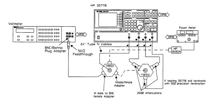
Figure 3-11. Absolute Accuracy and Flatness Test Set-Up  $(50\Omega)$
