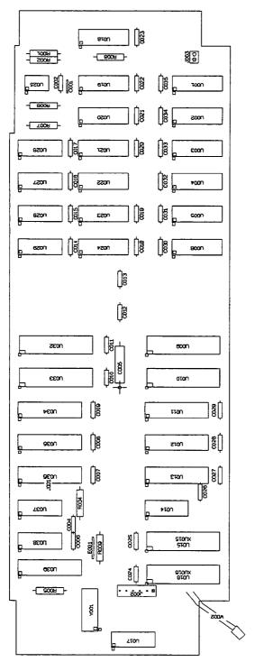
A84 Memory Circuit Component Locator Rev A
