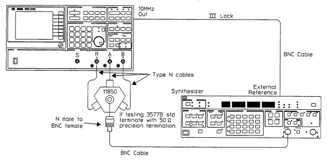
Figure 3-6. Dynamic Linearity (Magnitude vs. Phase)
