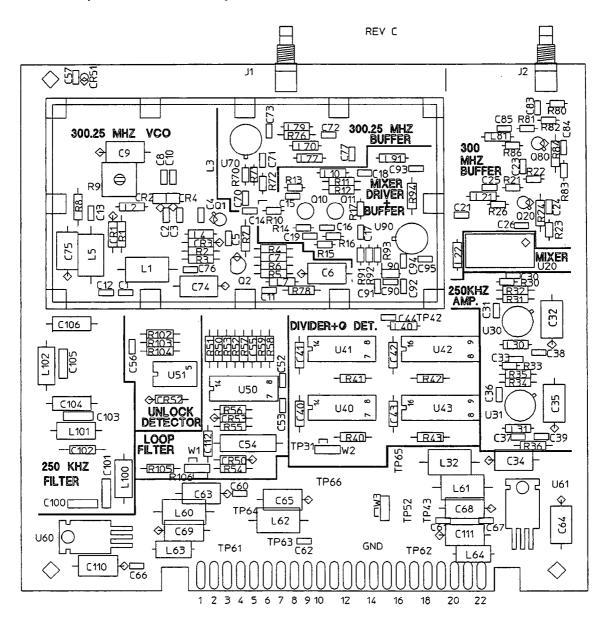
Figure 9-7. A5 Component Locator
