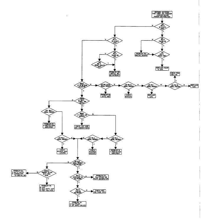
Figure 9-29. A81 X-Y-X Amplifier / Stroke Generator Troubleshooting Procedure
