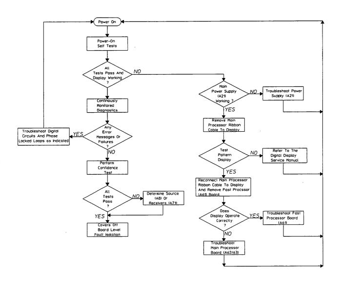
Figure 2-9. Fault Isolation Flow Diagram
