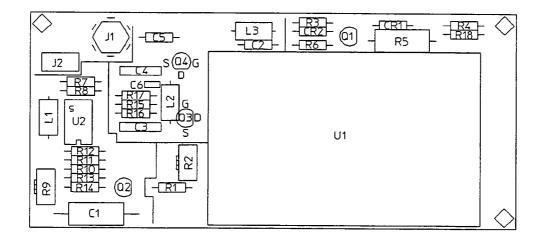
Figure 9-22. A31 Component Locator
