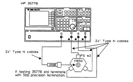
Figure 3-7. Calibration of Transmission Loss
