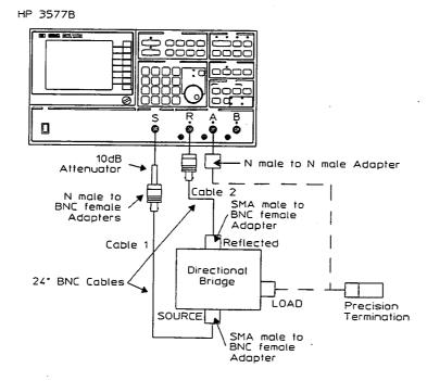
Figure 3-13. Receiver Return Loss Test Set-Up
