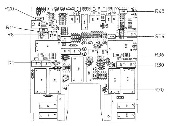
Figure 5-18. A81 Adjustment Locations for Stroke Generator and Stroke Length
