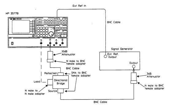
Figure 3-2. On Carrier Return Loss Test Set-Up
