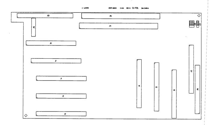
Figure 9-20. A20 Component Locator
