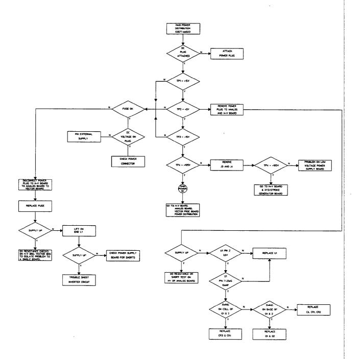
Figure 9-31. A83 Low Voltage Power Supply Troubleshooting Procedure
