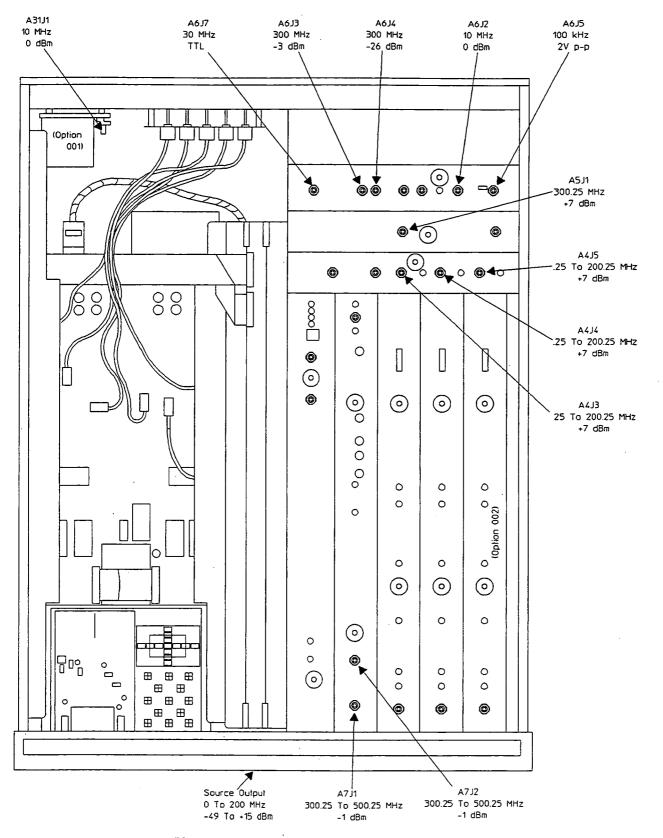
Figure 2-2. Fault Isolation Test Signal Locations
