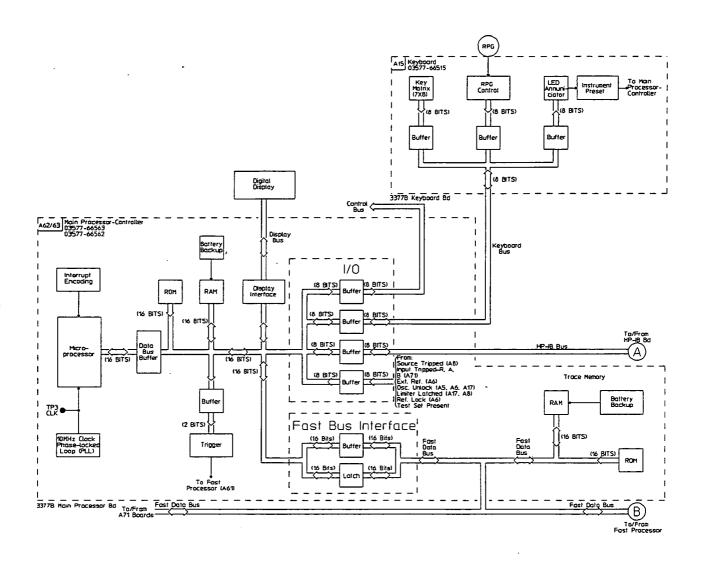
Figure 2-7. HP 3577B Functional Block Diagram, (A15/A62/63) Part 5 of 6
