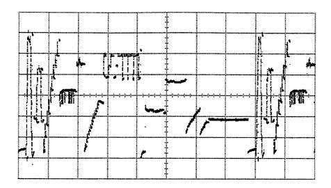
Figure 5-29. X-Amplifier Auxiliary Output Vertical attenuator = 200 mV/Div Sweep = 2 ms/Div
