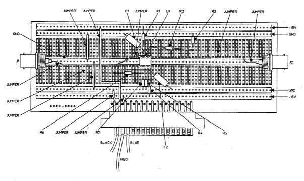
Figure 3-4. Suggested Layout for Buffer Amplifier
