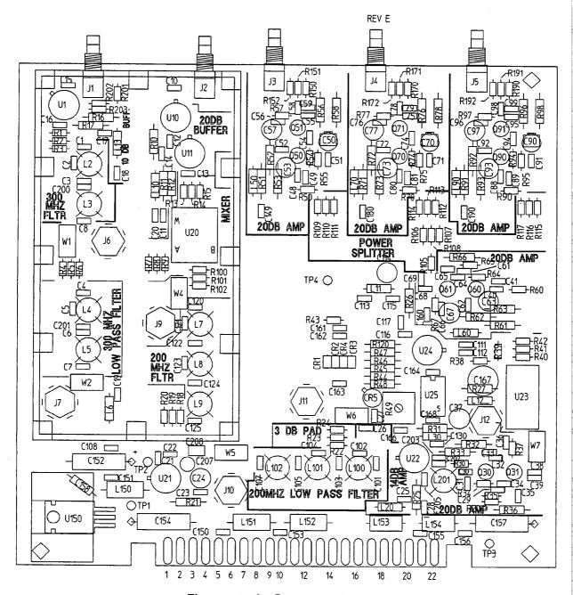
Figure 9-6. A4 Component Locator
