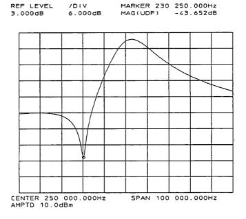
Figure 5-1. Input 250kHz Filter Frequency Response
