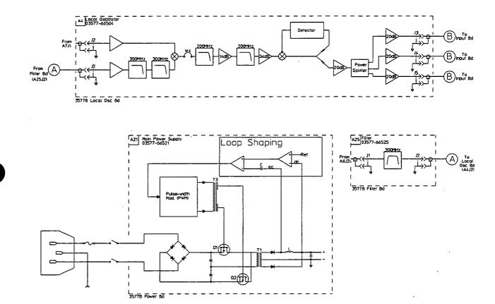
Figure 2-5. HP 3577B Functional Block Diagram, (A4/A21) Part 3 of 6
