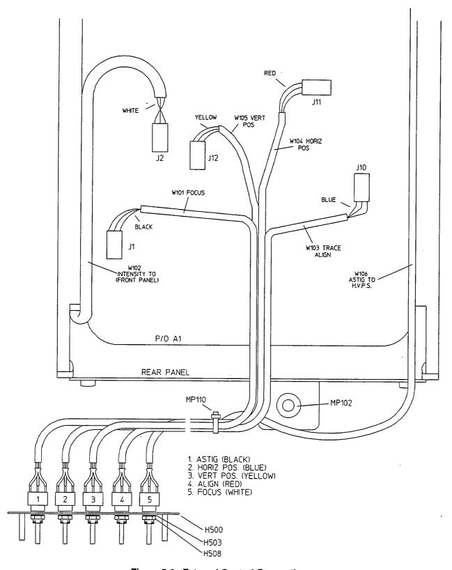
Figure 5-8. External Control Connections
