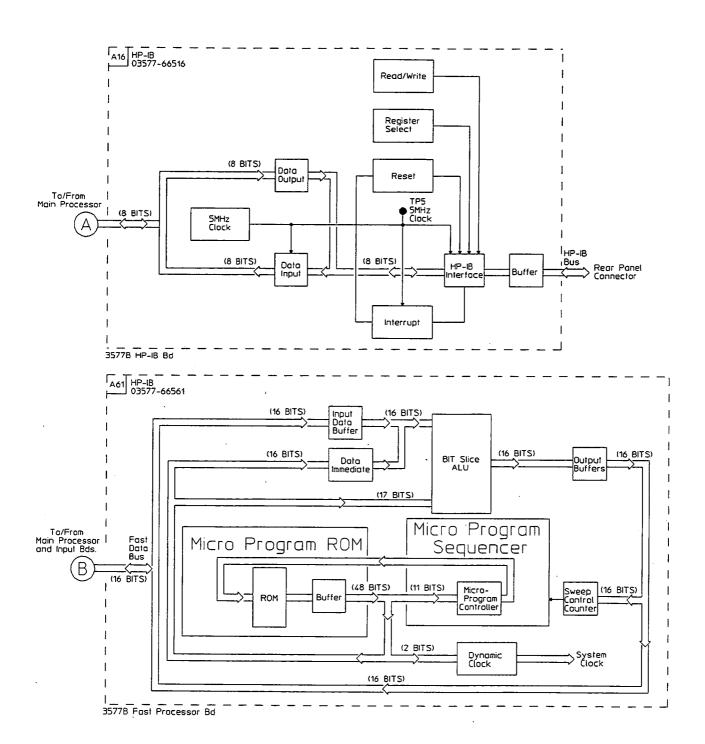
Figure 2-8. HP 3577B Functional Block Diagram, (A16/A61) Part 6 of 6
