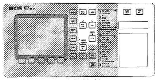
Figure 1-2. Front Panel Keys
