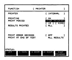
4. Set up the RESULTS display as shown opposite (on both HP 37717B's if end to end).
