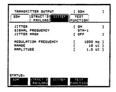
Select the required jitter MODULATING FREQUENCY and AMPLITUDE.
