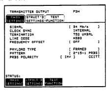
4. Set up the RECEIVE display STRUCTURED SETTINGS as shown below.
