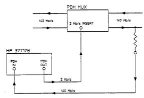
Figure 2-5. PDH Cross Multiplexer Testing
