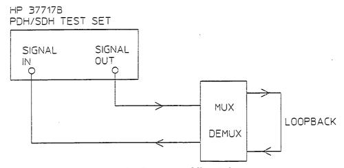
Figure 2-21. Frequency Offset Tolerance
