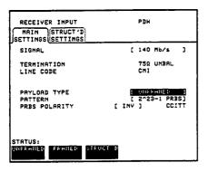
5. When the setting within a field is not enclosed in [ ] the field cannot be highlighted as no choice is available in the set up selected, as in TERMINATION and LINE CODE above.
