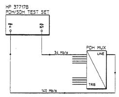
Figure 2-9. Structured PDH Jitter Tolerance Test
