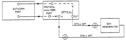
Figure 2-17. DCC Testing
