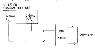
Figure 2-8. Frequency Offset Tolerance
