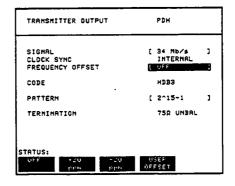
3. Select TX CLOCK OFFSET [+20ppm] and check that the Error Count and Error Ratio results are unchanged.
