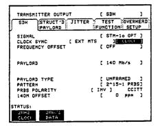
The CLOCK SYNC selection determines the synchronization source for the TRANSMIT clock. If [EXT MTS] is selected a 2 Mb/s reference must be connected to the front panel 2M REF IN port. The format can be CLOCK or DATA.
