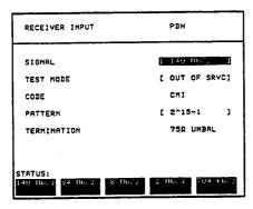
5. When the setting within a field is not enclosed in [ ] the field cannot be highlighted as no choice is available in the set up selected, as in CODE and TERMINATION above.
