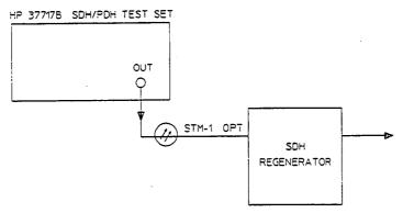
Figure 2-24. Optical Clock Recovery Stress
