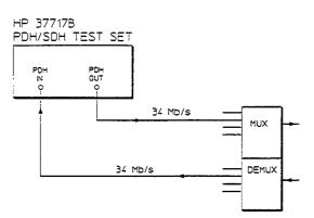
Figure 2-10. Unstructured PDH Jitter Tolerance Test
