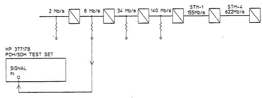
Figure 2-7. Frequency Measurement
