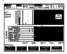
3. For more detailed inspection of the bar graph, position the cursor centrally within the area of interest using and and select ZOOM IN to reduce the time axis to 15 MINS/BAR. This is only possible if the graphics results were stored with a STORAGE resolution of 1 SEC, 1 MINS or 15 MINS.
