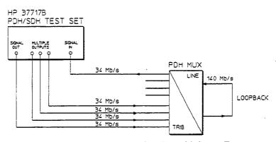
Figure 2-12. Unstructured PDH Multiplexer Test
