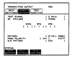
3. Set up the RECEIVE MAIN SETTINGS display as shown below.
