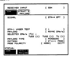
4. Set up the OTHER display, PRINTER function, as shown below.
