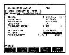
4. When a field has more than five choices, as in PATTERN above, a softkey labelled MORE is provided. When MORE is chosen the remainder of the menu is revealed as shown below.
