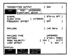
3. Set up the TRANSMIT TEST FUNCTION display as shown below.
