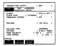
2. Set up the TRANSMIT TEST FUNCTION display as shown opposite.
