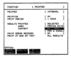
CONTENT [ER & ANAL] provides both BER and Analysis results at the end of each Print Period and at the end of the test period.
