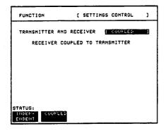
Any settings change made on the TRANSMIT or RECEIVE displays will automatically occur on the other.
