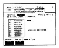
All section overhead bytes are monitored and displayed as shown below.
