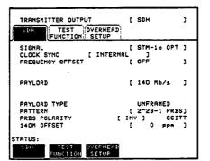
The CLOCK SYNC selection determines the synchronization source for the TRANSMIT clock.
