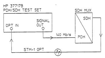
Figure 2-25. Payload Mapping
