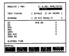
The following error results are available on the RESULTS display during the test period:
