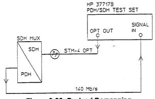
Figure 2-26. Payload Demapping
