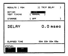
The delay measurement range is up to 2 seconds. The Resolution varies according to the received rate:
