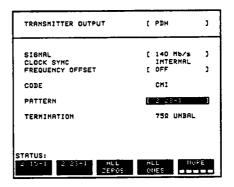
4. When a field has more than five choices, as in PATTERN above, a softkey labeled MORE is provided. When MORE is chosen the remainder of the menu is revealed as shown below.
