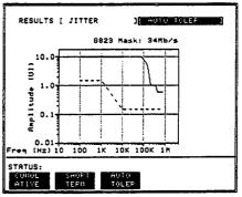
If Option 1CW, RS-232-C Remote control, or Option 1A8, HP-IB Remote Control, is fitted the Jitter Tolerance Mask results can be logged to an External printer (See Connecting an HP 550C DeskJet Printer). View the Jitter Tolerance results on the (RESULTS) display and press (RESULTS).
