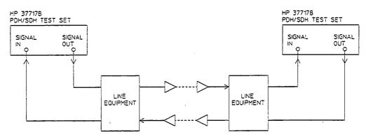
Figure 2-3. End-to-End Test
