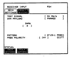
The required 34 Mb/s test signal is selected under 34Mb.
