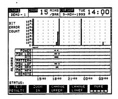
For further reduction of the time axis, to 01 MINS/BAR or 01 SECS/BAR, position the cursor centrally within the area of interest and select **Z00M** IN until the required time axis is obtained.
