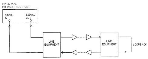
Figure 2-4. Loopback Test
