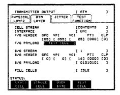
For BER testing select CROSS CELL or SINGLE CELL and required PRBS.
