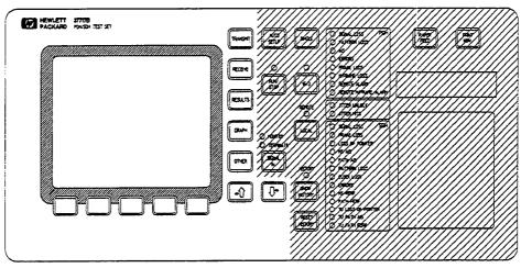
Figure 1-1. HP 37717B Front Panel
