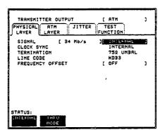
THRU MODE can be used for In-Service monitoring.
