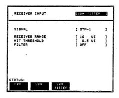
If Jitter filtering is required select from the softkey menu.
