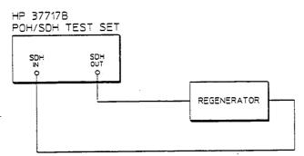
Figure 2-22. Jitter Transfer Test
