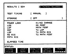
ALARM SECONDS are displayed but any of the other results can be selected from the softkey menu without affecting the measurement.
