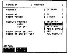
WHEN [PERIOD EC>0] ensures results are not logged on the printer when a print period is error free.
