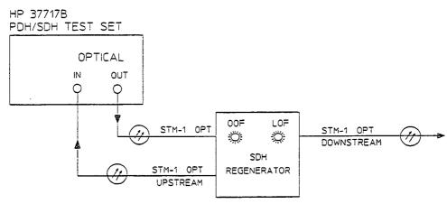
Figure 2-19. Frame Synchronization
