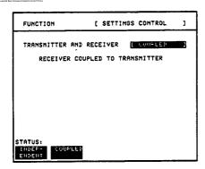
Any SDH settings change made on the TRANSMIT or RECEIVE displays will automatically occur on the other.
