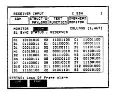
If any abnormal behavior is observed on a particular path or section overhead byte, or an associated group of bytes (3XA1,3XA2; D1 - D3) the RECEIVE TEST FUNCTION display of OVERHEAD CAPTURE can be used to "zoom" in on the suspect byte, or bytes, on a frame by frame basis.
