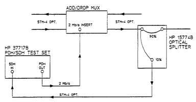
Figure 2-15. Add/Drop Multiplexer Testing
