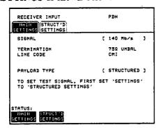
4. Set up the (RECEIVE) display STRUCTURED SETTINGS as shown below.
