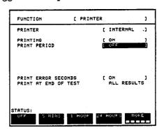
When making long term out-of-service bit error measurements it is often desirable only to log results when an error has occurred.
