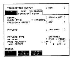
4. Set up the TRANSMIT TEST FUNCTION display as shown below.
