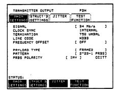
2. Select TRANSMITTER OUTPUT SETTINGS [JITTER] and set up the display as shown below.
