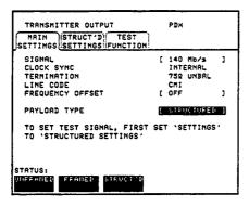
2. Set up the TRANSMIT STRUCTURED SETTINGS display as shown below.
