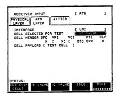
CELL SELECTED FOR TEST allows filtering of the cells of interest.
