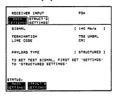
4. Set up the RECEIVE STRUCTURED SETTINGS display as shown below.
