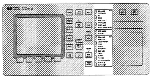
Figure 1-3. Front Panel Keys
