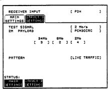
2M PAYLOAD Framing selection should match that of the network equipment.
