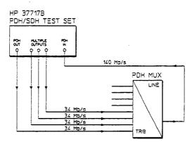
Figure 2-11. Structured PDH Multiplexer Test
