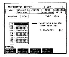
5. Selection of CRC7 MESSAGE allows the user to program the message content of the J1 byte with up to 15 ASCII characters (padded out with ASCII Null characters if necessary) followed by a frame marker byte with CRC7.
