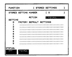
The recalling of factory default settings will configure the instrument in a defined state. One important feature of the factory default settings is that the Graphics Store capability is turned off. This prevents the possibility of any previously stored graphics data being discarded.
