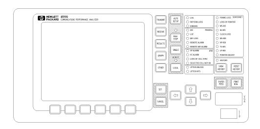
**AUTO SETUP** The test set attempts to match the settings to the received signal.
