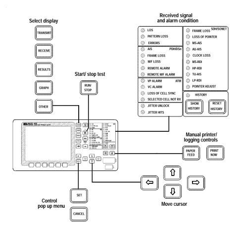
The operator interface is provided by the display and the front panel keys.
