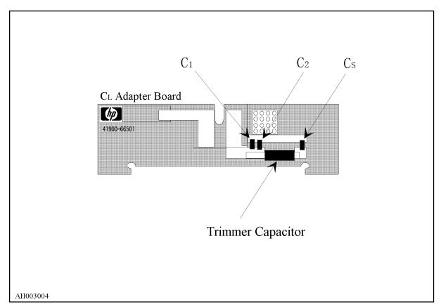
Figure 3-3.  $C_1$ ,  $C_2$ ,  $C_8$  Location
