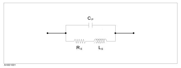
Figure 1-1. Circuit model of the calibration standards
