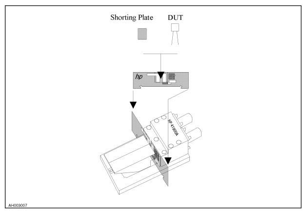
Figure 3-5.  $C_L$  Adapter Board Insertion
