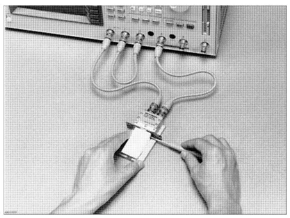
Figure 3-6. Load Capacitance Adjustment
