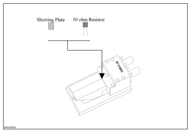
Figure 3-4. SHORT and LOAD Calibration
