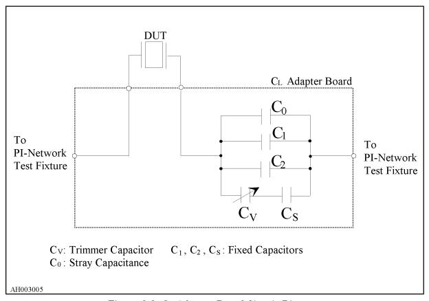
Figure 3-2. C<sub>L</sub> Adapter Board Circuit Diagram
