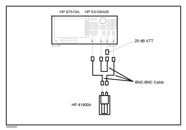
Figure 3-1. Connecting the 41900A to the 87510A, E5100A/B
