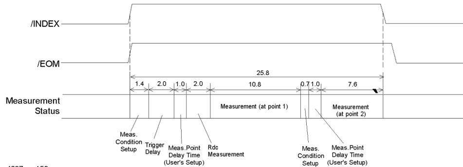
**Measurement Data Transfer Time through GPIB (Typical)**
