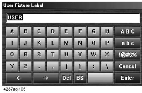
**Step 5.** Enter the label (name) of the newly registered test fixture in the label space at the top of the dialog box.
