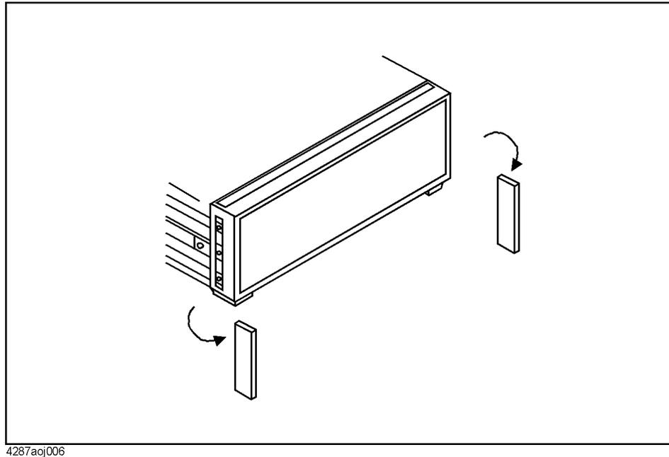
**Step 3.** Use the included screws to mount the two rack-mounting flanges (locking side plates) on the sides of the Agilent 4287A front panel frame.
