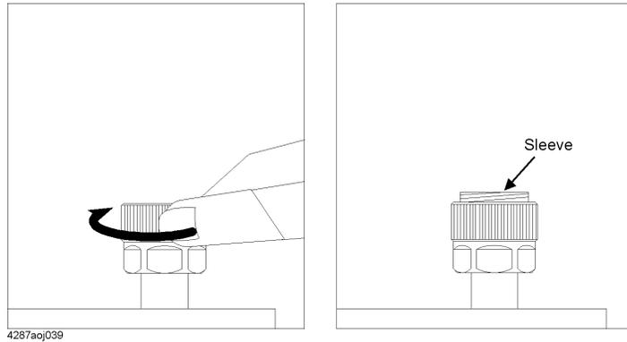
**Step 2.** Firmly connect the open standard (0 S) to the 7-mm terminal on the test head by turning it clockwise as viewed from the top (Figure 6-7).
