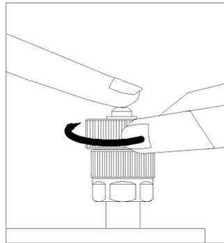
**Step 2.** Click the **SHORT** button in the calibration window and measure the short calibration data.
