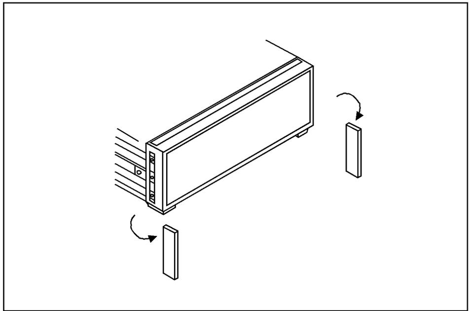
**Step 3.** Use the included screws to mount the two handles on the sides of the Agilent 4287A front panel frame.
