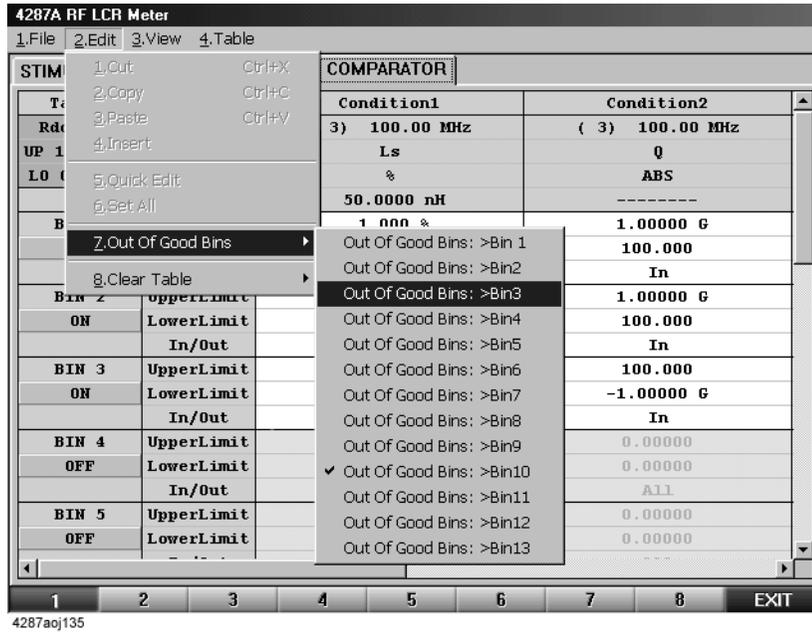
The GOOD BINS line is drawn between BIN 3 and BIN 4 as shown in Figure 8-33. In accordance with this setting, measurement results that do not meet the conditions set for BIN 1 to BIN 3 are judged to be OUT OF GOOD BINS.
