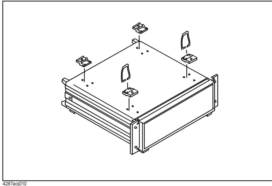
Step 5. Mount the Agilent 4287A on the rack.
