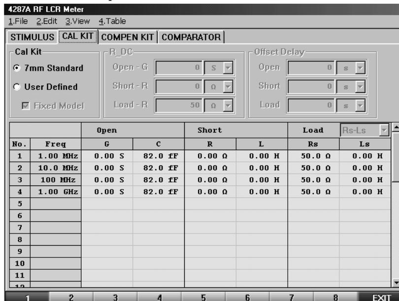
**Step 2.** Specify the table number to define a calibration kit by following the description in “How to specify table number for setup” on page 104.
