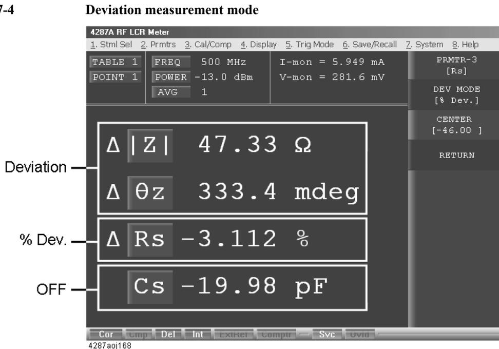
How the instrument displays measurement results differs according to the modes, as summarized in the table below.
