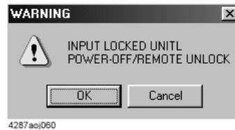
**Step 3.** Press the **OK** button in the dialog box to simultaneously lock the front panel keys, keyboard and mouse.
