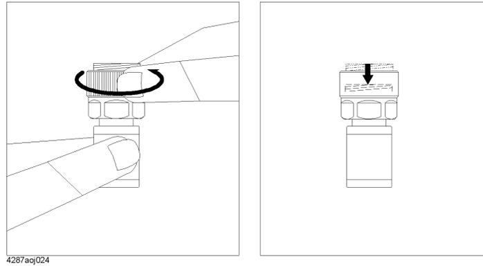
**Step 3.** While pressing the load standard (50  $\Omega$ ) from above, turn the connector nut clockwise and securely connect it to the 7-mm terminal (Figure 3-21).
