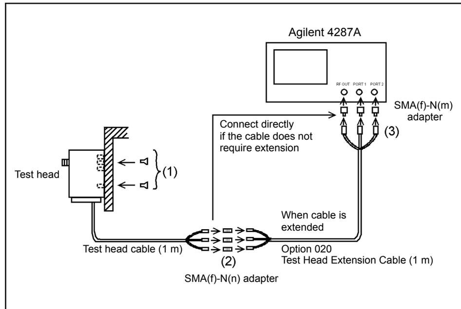
**Step 1.** Use one or more of the four screw holes in the test head to secure the test head to a handle or other appropriate location (Figure 2-15 (1)).
