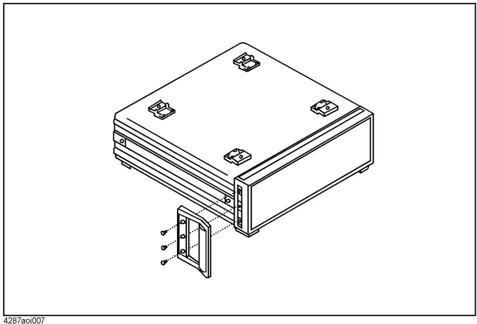
**Step 4.** Attach the included modified trim strip in order to cover the front panel locking screws.
