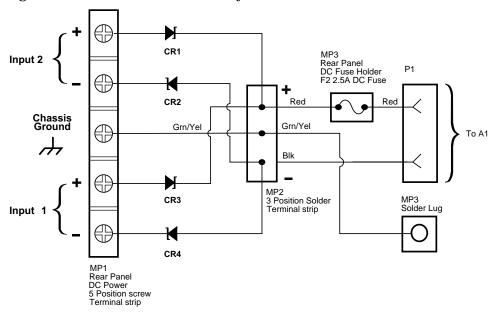
Figure 2-1. DC Input 1 and 2 Power Steering Schematic (48V Subpanel Assembly, part number 05071-60277)
