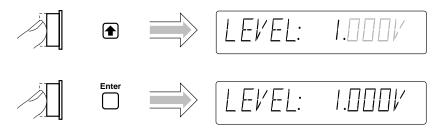
Channel 1's trigger level is now set to +1V.
