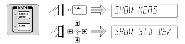
Updating the SHOW configuration caused Stats to be enabled. The Stats indicator is now lit.
