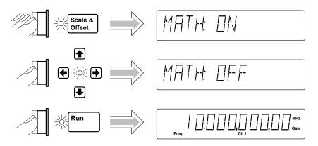
The Counter is now making measurements without the scale/offset values calculated into the measurements.
