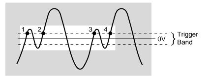
The Counter should now be triggering as determined by the sensitivity level, and displaying the input signal's frequency if the input signal peak-to-peak voltage is large enough for the selected sensitivity level.
