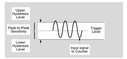
Signal will not generate a count because the trigger level is set below the midpoint of the signal, causing the lower hysteresis level to not be crossed. The sensitivity specification is given in terms of volts rms for applications that involve measuring a sine wave signal, though it should be noted that a different waveform with the same rms voltage may not trigger a count.
