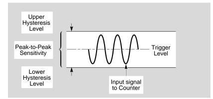
Signal will not generate a count because the peak-to-peak amplitude of the signal is insufficient.
