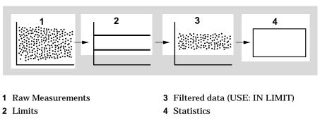
Figure 1-4. Filtering Data Before Statistical Computation
