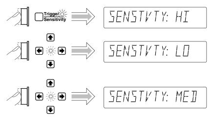
Refer to the sub-section titled "To Use the Trigger/Sensitivity Key to Adjust Counter's Trigger Voltage and Sensitivity Levels" in Chapter 2 for more information about sensitivity, if needed.
