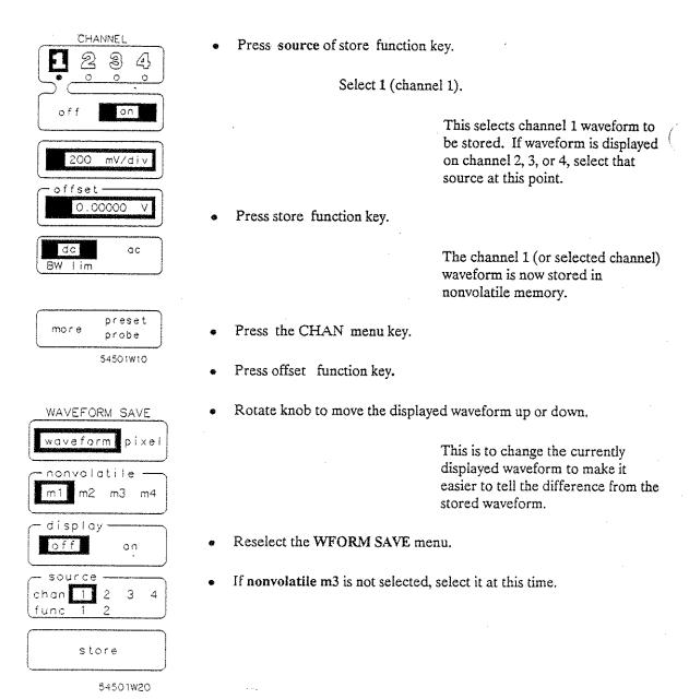
Press display function key in the waveform save menu.
