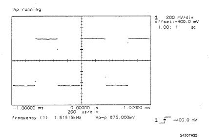
If another measurement is made, after the screen is full, it is placed on the bottom display line and the top set of measurements are erased from the display.
