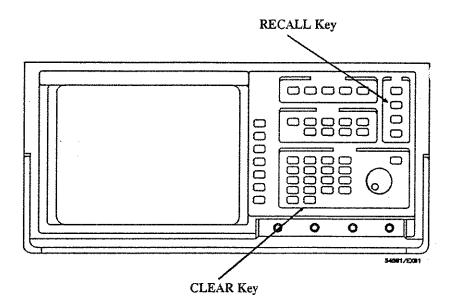
Basic oscilloscope setups are performed in this chapter. The setups are performed automatically and manually. Generally, the automatic setup is used on an unknown signal or signals, then the oscilloscope is adjusted manually for fine-tuning.
