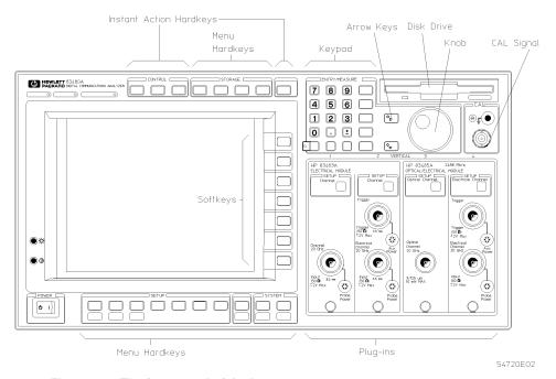
Figure 1-1. The front panel of the instrument
