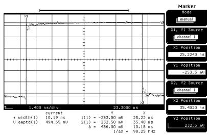
Figure 2-5. Signal automatic measurements
