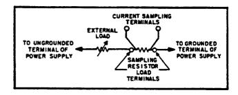
Figure 5-2. Output Current Measurement Technique
