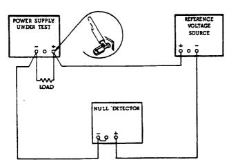
Figure 5-3. Differential Voltmeter Substitute, Test Setup
