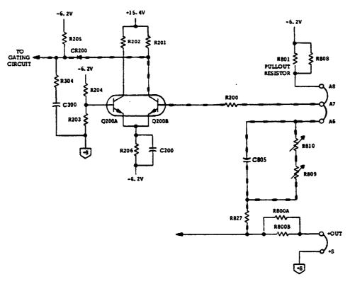
Figure 4-7. Constant Current Input Circuit, Simplified Schematic
