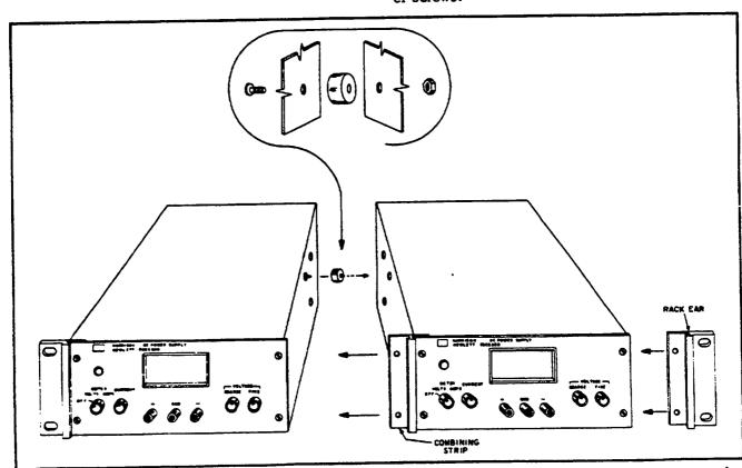
Figure 2-1. Rack Mounting, Two Units
