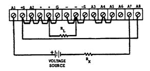
Figure 3-6. Remote Voltage Programming (Constant Current)
