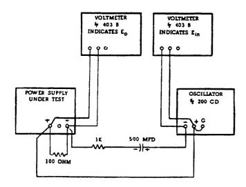
Figure 5-9. Output Impedance, Test Setup
