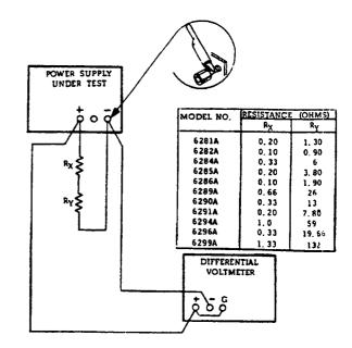
Figure 5-5. Load Regulation, Constant Voltage
