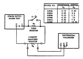
Figure 5-4. Output Current Test Setup
