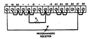
Figure 3-5. Remote Resistance Programming (Constant Current)
