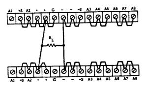
Figure 3-10. Normal Parallel Connections
