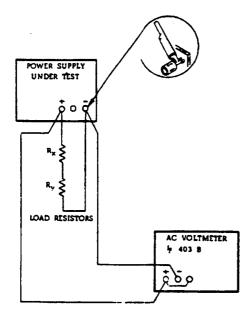
Figure 5-6. Ripple and Noise, Constant Voltage
