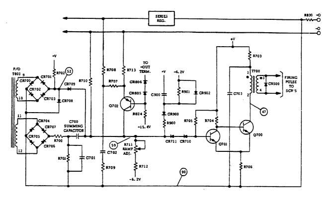
Figure 4-4. SCR Control Circuit, Simplified Schematic
