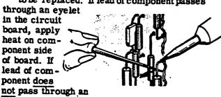
eyelet, apply heat to conductor side of board.
