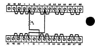
Figure 3-8. Normal Series Connections
