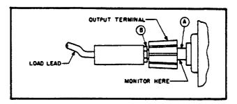
Figure 5-1. Front Panel Terminal Connections
