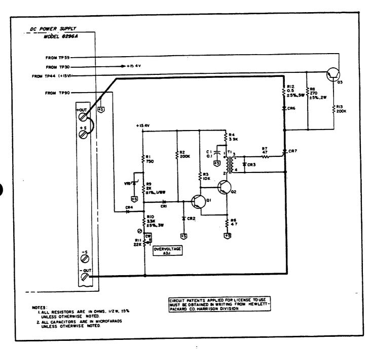
Figure A-1. Model 6296A Overvoltage Protection Crowbar
