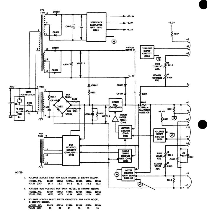
Figure 4-2. Simplified Schematic
