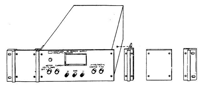
Figure 2-2. Rack Mounting, One Unit
