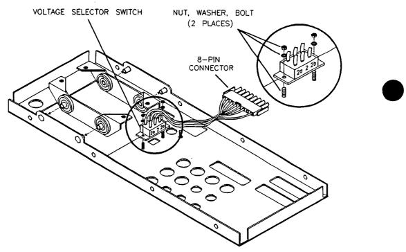
Figure 7-17. Voltage Selection Switch Removal
