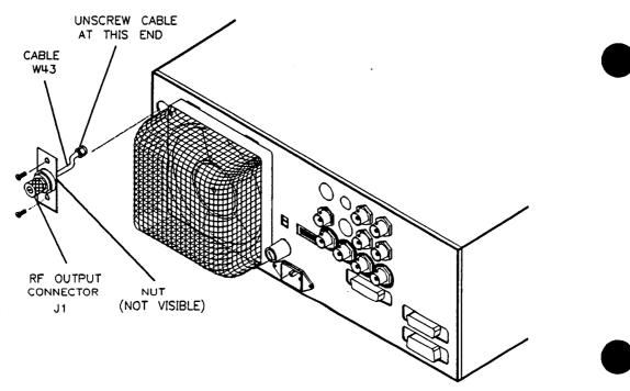
Figure 7-23. Removing RF Output Connector
