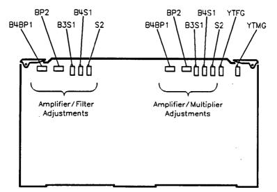
Figure 3-15. A12 Assembly Potentiometer Locations
