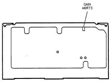
Figure 3-9. IF Gain Adjustment Location
