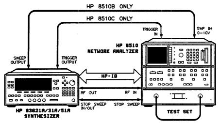
Figure 2-3. Swept Frequency Accuracy Setup
