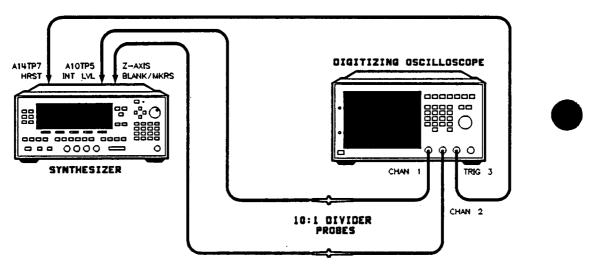
Figure 3-20. Low Power SRD Bias Adjustment Setup
