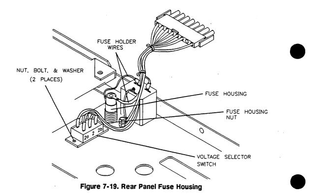
Note: To reassemble, add 3/8 in. shrink tubing to each wire before soldering. Then perform the above steps in reverse order.
