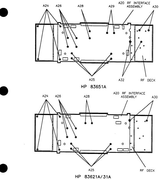
Figure 7-29. RF Deck Screw Locations
