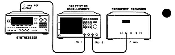
Figure 3-1. 10 MHz Standard Adjustment Setup
