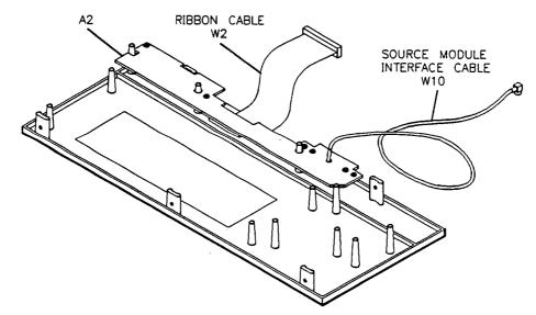
Figure 7-5. Front Panel Coaxial and Ribbon Cable Locations
