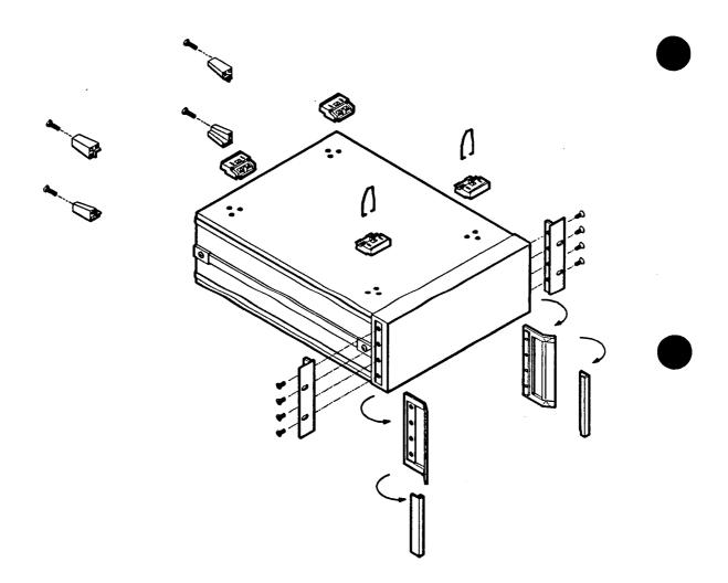
Figure 12-7. Rack Mount Flanges for Synthesizers with Handles Removed
