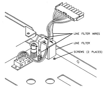
Figure 7-20. Line Filter Removal
