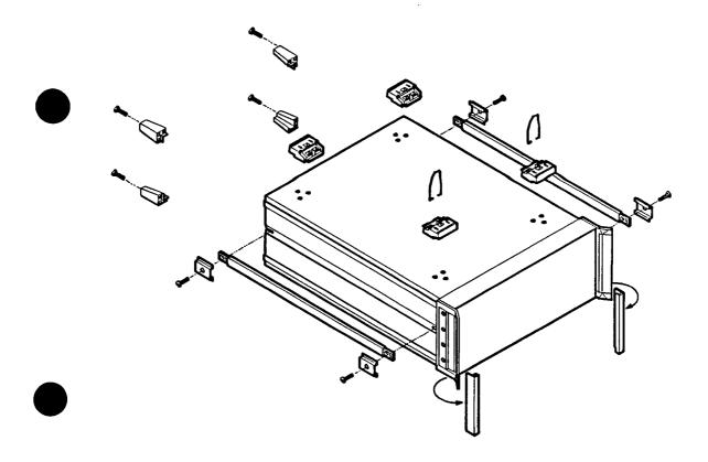
Figure 12-5. Removing the Side Straps and Feet
