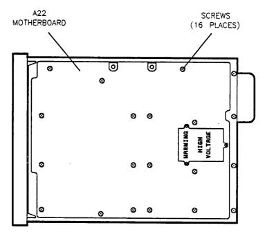
Figure 7-42. Motherboard Screws
