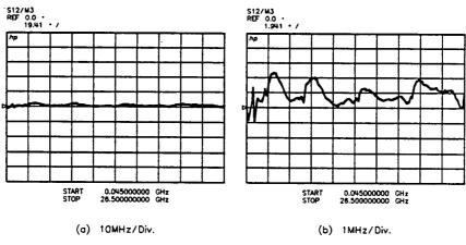
Figure 2-4. Bandswitch Transition Location
