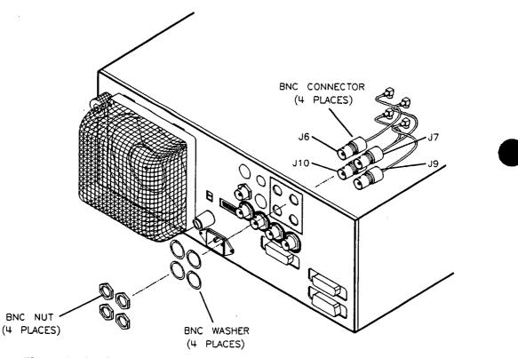
Figure 7-10. J6, J7, J9, and J10 Rear Panel BNC Connector Locations
