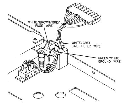
Figure 7-18. Fuse, Line Filter, and Ground Wires
