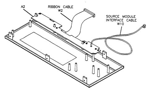
Figure 7-35. Front Panel Coaxial and Ribbon Cable Locations
