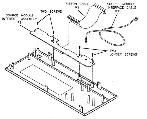
Figure 7-6. Source Module Interface Removal
