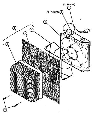
Figure 9-7. Rear Panel Fan Assembly
