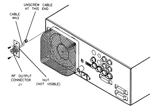
Figure 7-11. Removing RF Output Connector
