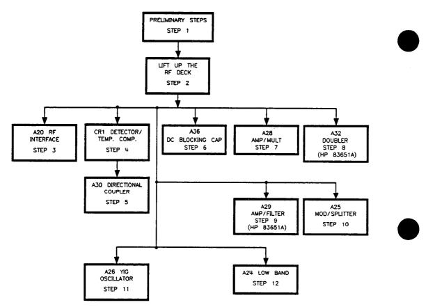
Figure 7-22. RF Deck Disassembly Flowchart
