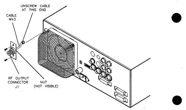
Figure 7-36. Removing RF Output Connector
