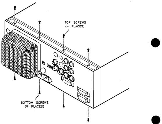
Figure 7-37. Rear Panel Removal
