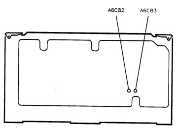
Figure 3-8. Sampler Match Adjustment Locations
