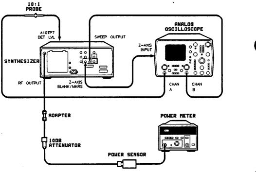
Figure 3-18. Amplifier/Filter Adjustments Setup
