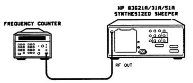
Figure 2-1. CW Accuracy Test Setup
