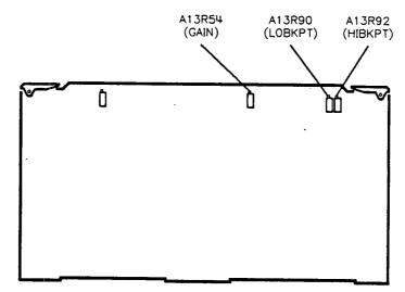
4. Adjust A13R54 (see Figure 3-12) to center the "needle" on the display.
