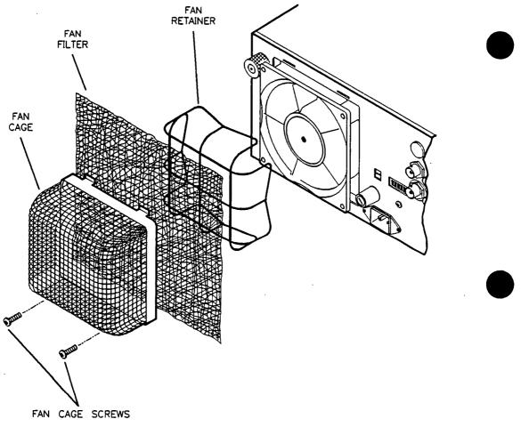
Figure 10-1. Removing the Fan Filter
