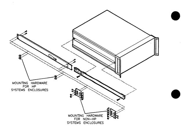
Figure 12-6. Chassis Slide Kit
