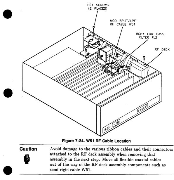
6. Carefully pull out the RF deck and rest it on the side of the instrument.
