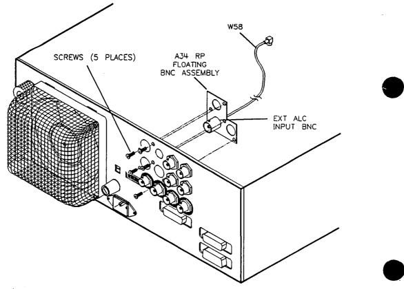
Figure 7-21. Ext ALC Input BNC Connector Removal
