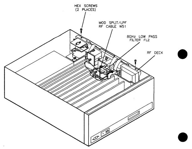
Figure 7-40. W51 RF Cable Location
