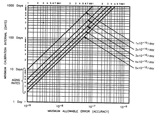
Figure 3-3. Accuracy Versus Adjustment Interval
