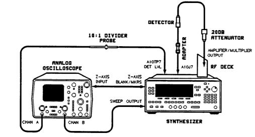
Figure 3-14. Amplifier/Multiplier Adjustments Setup
