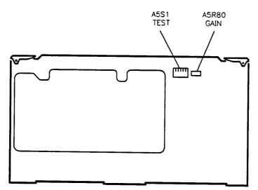
Figure 3-13. Switch and Adjustment Locations
