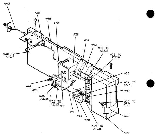
Figure 7-28. RF Deck Cable Locations - HP 83621A/31A
