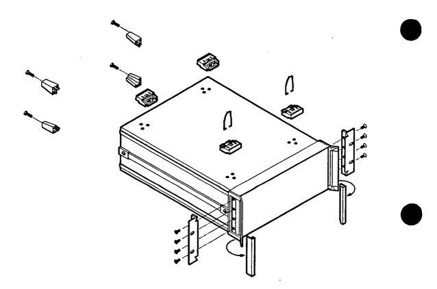
Figure 12-8. Rack Mount Flanges for Synthesizers with Handles Attached
