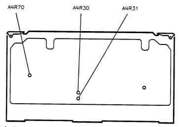
Figure 3-6. Fractional-N Reference and API Spurs Adjustment Locations
