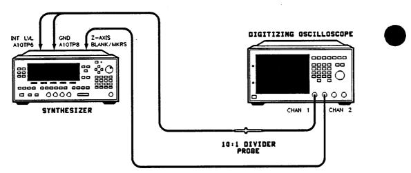
Figure 3-23. Modulator Offset and Gain Adjustment Setup
