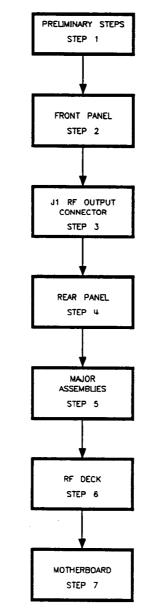
Figure 7-32. Motherboard Disassembly Flowchart
