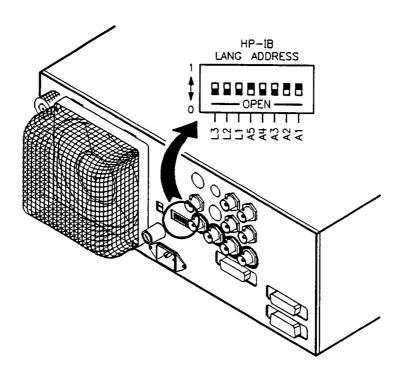
Figure 5-1. HP-IB Switch with TMSL Setting
