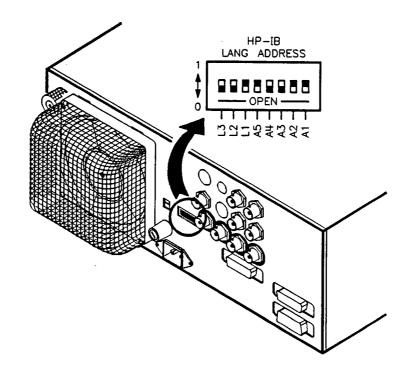
Figure 12-2. Rear Panel HP-IB Switch
