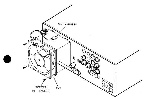
Figure 7-9. Fan Removal
