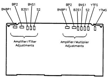
Figure 3-19. A12 Assembly Potentiometer Locations
