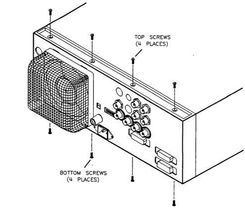
Figure 7-12. Rear Panel Removal
