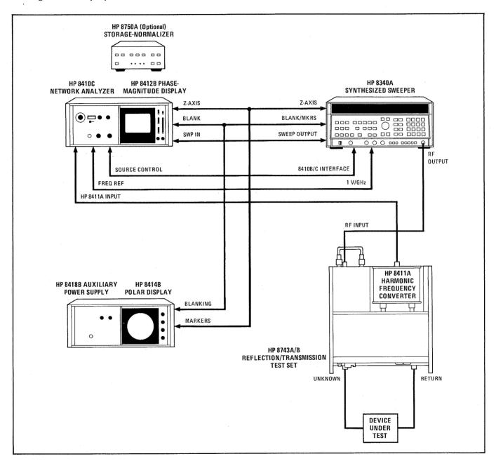
Figure 1. HP 8340A Connections to HP 8410C
