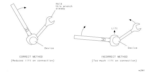
2. Hold the torque wrench lightly, at the end of the handle only (beyond the groove). See Figure 3-8.
