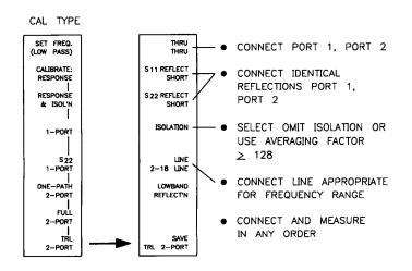
TRL 2-PORT calibration type uses multiple measurements of the thru connection, identical reflection standards at each port, and a transmission line of appropriate length and impedance to measure the error terms. If proper standards are available, this is the preferred technique due to fewer connections required and the potential for more accurate characterization of the error terms. More details of this calibration procedure are contained in other documentation supplied with the HP 8510 system.
