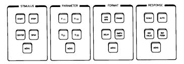
**Basic Measurement Functions - S/P/F/R.** Next, there are groups of keys for the measurement setup, measurement calibration, data presentation, and data output functions. The basic measurement and display functions are specified using keys in the STIMULUS, PARAMETER, FORMAT, and RESPONSE blocks.
