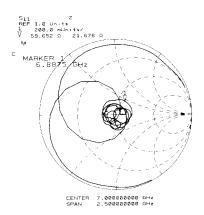
The S-parameters are measured in exactly the same way as described above. An S-parameter is always a complex coefficient consisting of a linear magnitude ratio and a phase angle, defined with the DUT embedded in a known characteristic impedance, usually 50 ohms. These figures show the reflection measurement viewed using the [LIN mkr on POLAR] format. The marker reads out the S-parameter directly.
