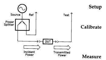
Insertion Loss and Gain are ratios of the output signal to the input signal. When set up as shown below, the results can be read directly in decibels.
