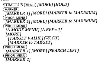
The markers are now at the -3 dB frequencies and the 3 dB bandwidth is displayed in the active function area.
