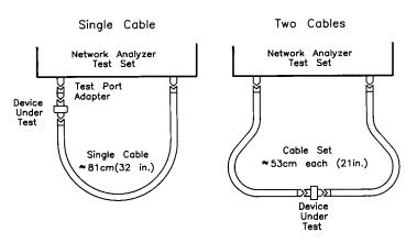
The point(s) at which the device under test is connected to the test set is called the Reference Plane(s). If cables are used to extend the test set port out to the device under test, the end of the cable is defined as the Port 1 and Port 2 reference plane. All measurements are made with respect to the reference plane(s).
