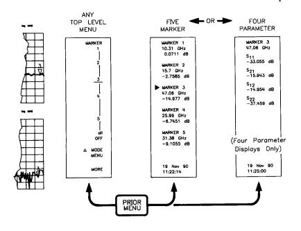
The five marker list can be selected for any display mode. The four parameter marker list can only be selected with a four parameter display.
