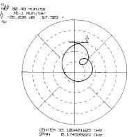
Twelve different display formats provide a comprehensive selection of useful presentations. The keys in the FORMAT block and displayed by FORMAT (MENU) also select the marker units shown by the active marker. This list shows the trace value and marker units for each of the standard format selections. Examples of how these formats are used for various reflection and transmission measurements are discussed in later chapters.
