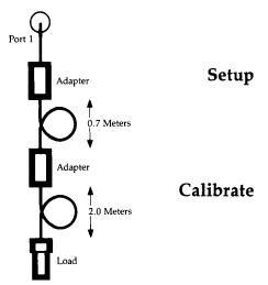
The test device is a pair of test cables shown in the figure, connected by one or two adapters to make things interesting. Terminate the end of the cable with a fixed load. Proceed as follows to measure this device.
