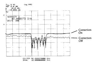
Accuracy in network measurements is greatly influenced by factors external to the network analyzer frequency conversion and signal processing steps. Parts of the measurement setup such as interconnecting cables and test sets all introduce variations in magnitude and phase that can distort the actual performance of the DUT. Because the magnitude and phase of the error is unknown, each error is assumed to have a cumulative effect of increasing the uncertainty of the measured data.
