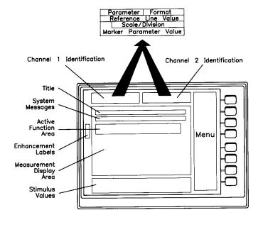
**CRT Display.** The front panel of the network analyzer is relatively simple. It is shown in full by the foldout at the end of this document. First, there is the CRT which presents the measurement results. This illustration shows the general areas for the measurement trace and for the various annotations which communicate to the operator.
