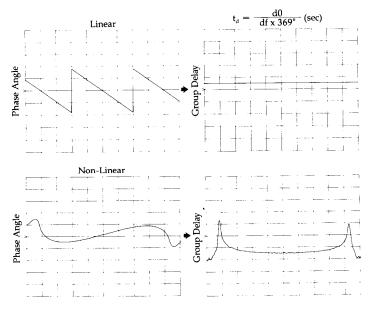
**Group Delay.** The phase linearity of many devices is specified in terms of group or envelope delay. This is especially true of telecommunications components and systems. After calibration, select (DELAY) to view the group delay of the DUT.
