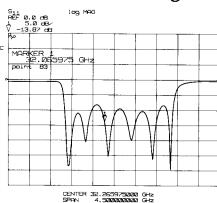
This figure shows the return loss of a filter in the LOG MAG format. A typical filter has a poor match (near 0 dB) outside the passband and a good match (large numerical) inside the passband. A large numerical value for return loss, for example —40 dB, corresponds to a small reflected signal (the reflected signal is 40 dB below the incident signal) just as a large value for insertion loss corresponds to a small transmitted signal.
