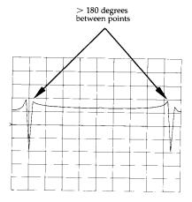
Group Delay Aperture. The minimum aperture is the frequency step between the phase measurements. You must choose this aperture when you set the frequency range and number of points so that there is no more that 180 degrees of phase shift between any of the frequency points. If there is more than 180 degrees of phase shift, the group delay trace will show a sudden discontinuity.
