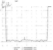
This figure shows the reflection measurement in terms of standing wave ratio, a unitless ratio of reflected to incident signal. SWR equal to one means that none of the incident signal is reflected.
