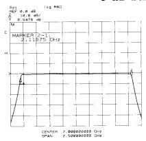
The marker search functions can be used to read the 3 dB bandwidth as follows:
