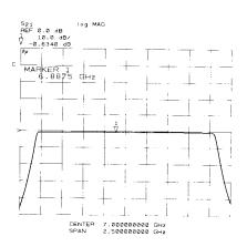
Calibration for insertion loss and gain sets the magnitude ratio to zero dB at all frequency points with the thru connection. After connecting the test device, a negative measured value indicates loss; a positive measured value indicates gain. This figure shows the insertion loss of a bandpass filter.
