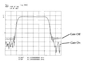
Time domain analysis also lets you remove individual parts of the time domain response to see the effect of potential design changes. We do this by mathematically "gating" out the undesired responses. In this example we see the effect of removing the leakage and triple travel responses using the gating feature. Press
