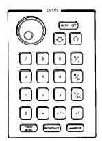
**Knob and Numeric Entry.** The value of the active function is changed using the ENTRY controls. The knob changes the function value in steps related to the current function value and the speed of the knob. The STEP keys change the active function value by a proportional increment each time the key is pressed. Enter a numeric value using the numeric, the decimal, and the +/- toggle, then pressing the appropriate units key.
