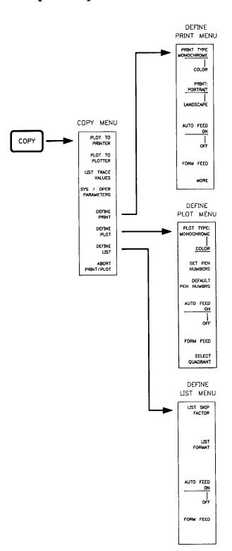
Measurement results can be output to a graphics printer, digital plotter, or a line printer using using selections in the COPY) menu structure. The HP 8510C adds two RS-232 ports for connection of hardcopy output devices. Moving the output devices from the 8510 system bus to the RS-232 ports may improve measurement throughput because since the RS-232 ports are fully buffered, the measurement can continue while the plot is being produced.
