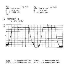
In the Dual Channel displays, as you make changes to the instrument state, notice that some settings are Coupled, meaning that the setting always applies to both channels, and others are Uncoupled, meaning that the setting applies only to the current selected channel. An example of the a function that is always coupled is Number of Points, on the Stimulus menu. An example of a function that is always uncoupled is Averaging, on the Response menu.
