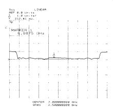
This figure shows the reflected signal viewed using the [LINEAR MAGNITUDE] cartesian format. In this format a reflection coefficient of 1.00 means that 100 percent of the signal is reflected. Inside the passband a value of 0.7 means that 70 percent of the signal is reflected.
