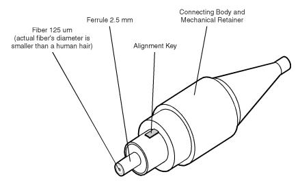
Figure 1-1. Basic components of a connector.
