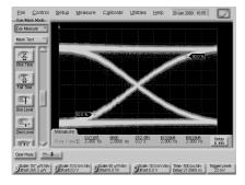
Once you are in Eye/Mask mode, press the Autoscale button. This ensures that an optimum eye diagram is displayed on the graticule. An optimum eye diagram consists of a full display of the eye in addition to portions of the waveform preceding and following the eye.
