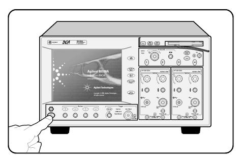
Press the power switch at the lower left-hand corner of the front panel.
