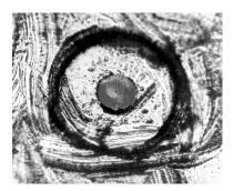
Figure 1-6. Damage from improper cleaning.
