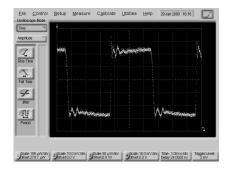
When you select the Oscilloscope mode, the measurement toolbars shown here appear. These measurement toolbars include measurements such as rise time, fall time, overshoot, and Vp-p. All measurements, with the exception of jitter, can be performed on any of the following sources: channels, waveform memories, and math functions. One of the above sources must be turned on in order to perform an oscilloscope measurement.
