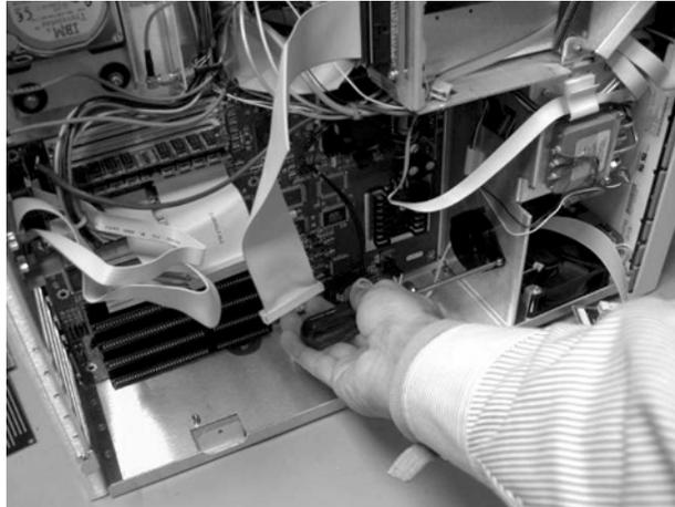
**Figure 4-38. Removing the Speaker Screw**
