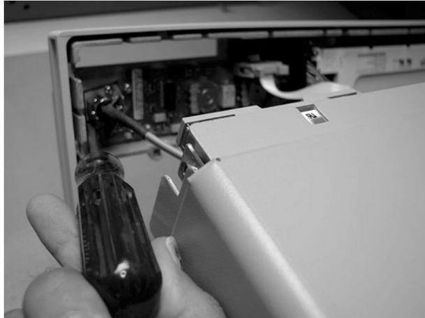
**Figure 4-9. Removing Screws that Secure the Cal Connector**
