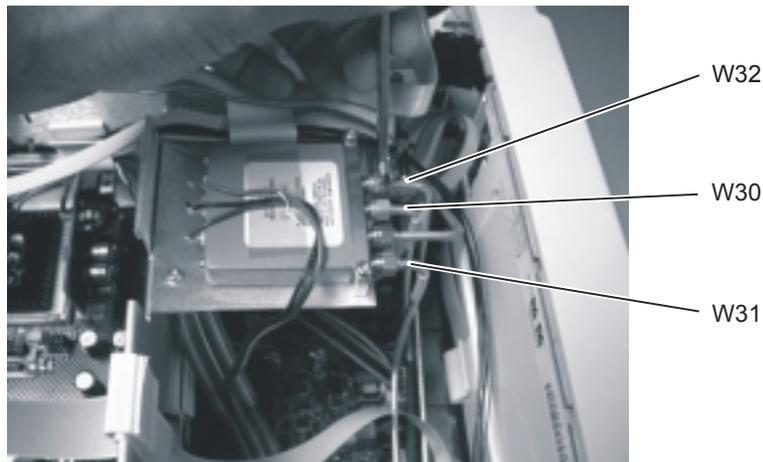
**Figure 4-48. Removing the Cables from the Coaxial Switch**
