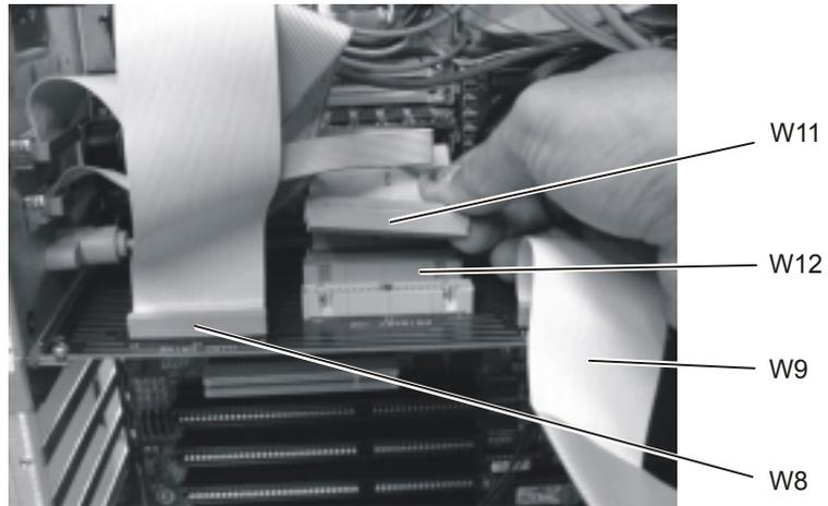
**Figure 4-46. W8, W9, W11, and W12 Cables**
