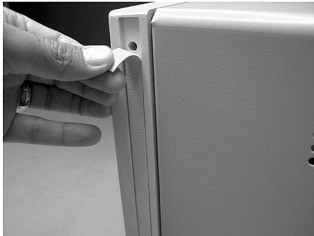
**Figure 4-6. Removing the Trim Strips**
