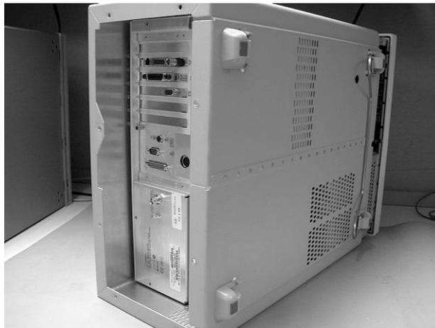
**Figure 4-5. Sliding Cover off Mainframe**
