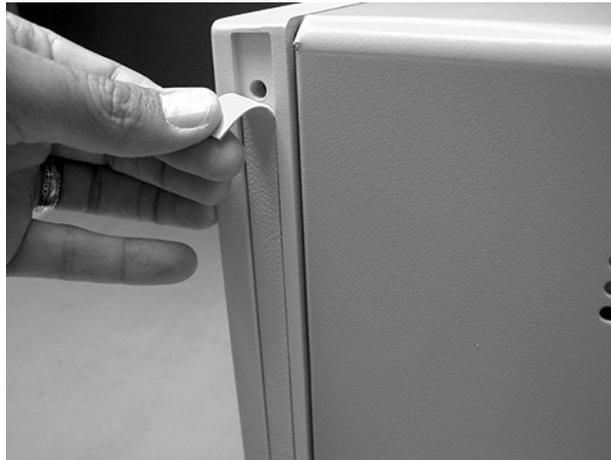
**Figure 4-26. Removing the Trim Strips**
