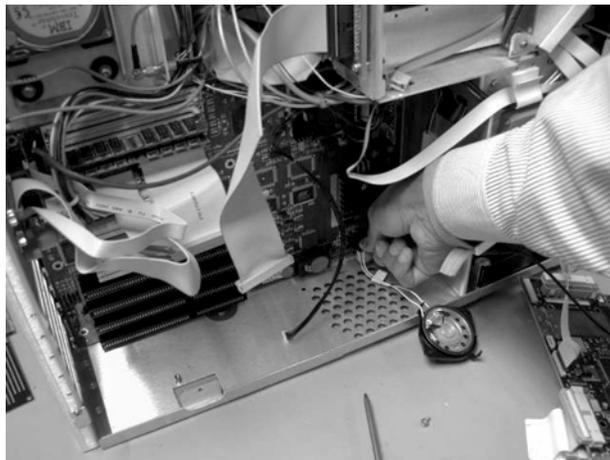
**Figure 4-39. Disconnecting the Speaker Cable**
