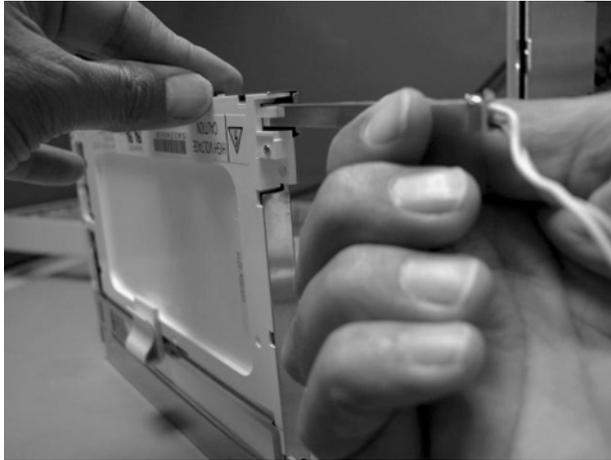
**Figure 4-20. Removing the Backlight**
