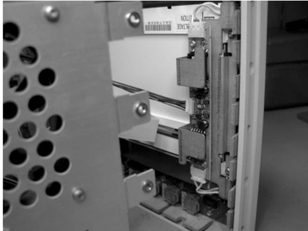
**Figure 4-28. Accessing the Inverter Board**
