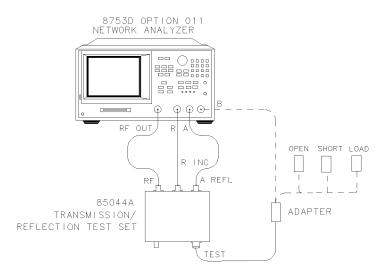
Figure 6-17. Receiver B Input Impedance Test Setup
