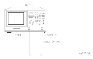
Figure 6-20. Receiver R Input Impedance Test Setup
