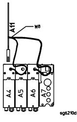
Figure 4-7. Connections for Substituting the R Sampler (A4)
