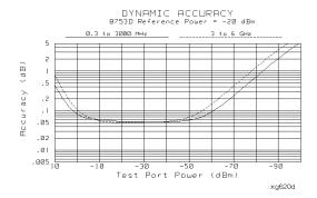
Figure 4-30. Receiver Magnitude Dynamic Accuracy
