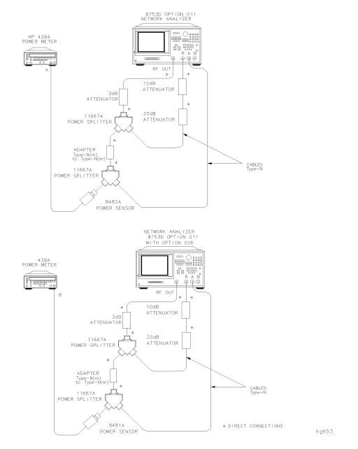
Figure 6-26. Channel A Magnitude Compression Test Setup
