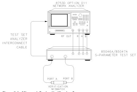
Figure 5-6. Mismatch Device Verification Setup
