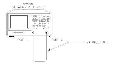
Figure 4-13. Test Port 1 Input Frequency Response Test Setup
