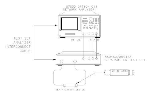
Figure 5-4. Connections for the 20 dB Verification Device
