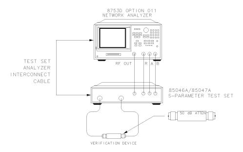
Figure 5-5. Connections for the 50 dB Verification Device
