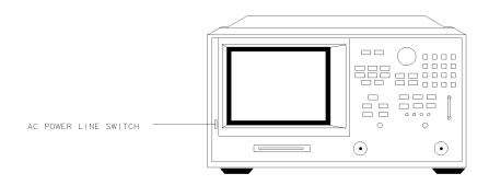
Figure 1-7. Turning on the Instrument
