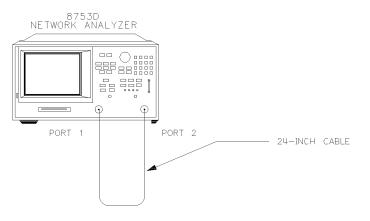
Figure 4-27. Test Port 2 Input Impedance Test Setup
