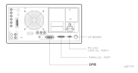
Figure 1-6. Rear Panel Peripheral Connections
