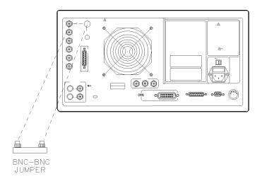
Figure 1-2. Jumper Cable Connection
