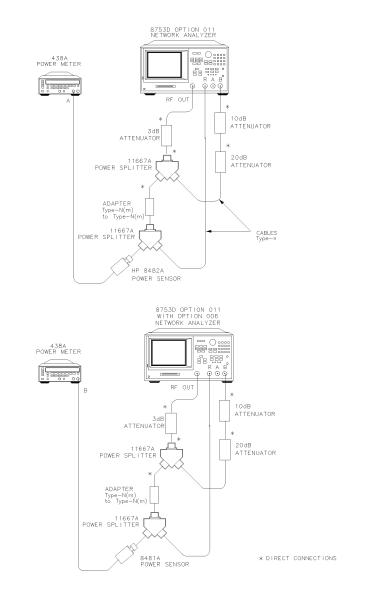
Figure 6-28. Channel R Magnitude Compression Test Setup
