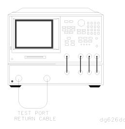
Figure 1-19. Transmission Mode Connections
