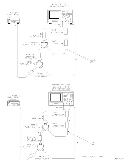
Figure 6-29. Channel A Phase Compression Test Setup
