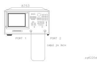
Figure 4-24. System Trace Noise Test Setup
