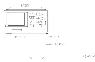
Figure 4-34. Test Port Magnitude Compression Test Setup
