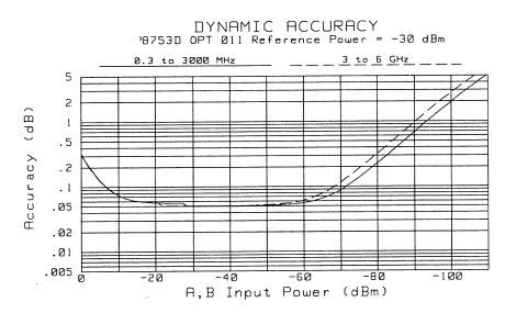
Figure 6-21. Receiver Magnitude Dynamic Accuracy
