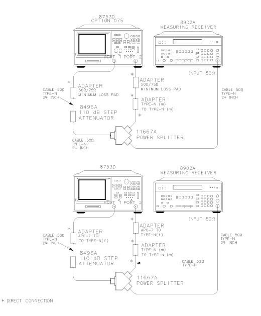
Figure 4-31. Test Port 2 Dynamic Accuracy Test Setup
