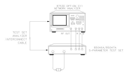
Figure 5-3. Transmission Calibration Setup
