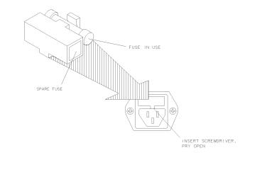
Figure 7-1. Line Fuse Removal and Replacement
