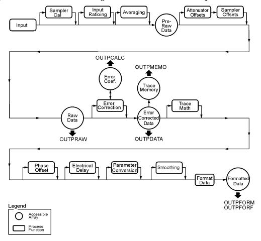
Figure 6-1. The Data-Processing Chain For Measurement Outputs
