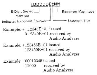
In general, do not issue numeric data with more significant digits than can be displayed on the Audio Analyzer's five-digit left display.
