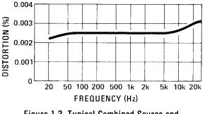
Figure 1-3. Typical Combined Source and Analyzer Residual Distortion
