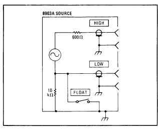
Simplified Schematic of the Audio Analyzer Source Output
