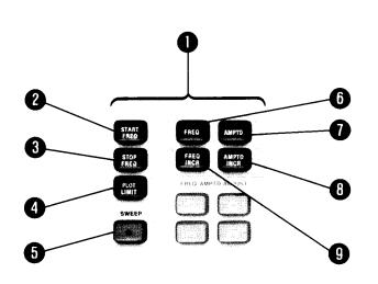
Source Prefix Keys. In addition to the functions described, the following keys are used to prefix numeric entries for the specified functions: START FREQ, STOP FREQ, PLOT LIMIT, FREQ, FREQ INCR, AMPTD, AMPTD INCR. The same specified function can be changed repeatedly without repressing the same prefix key as long as no other prefix key is pressed.
