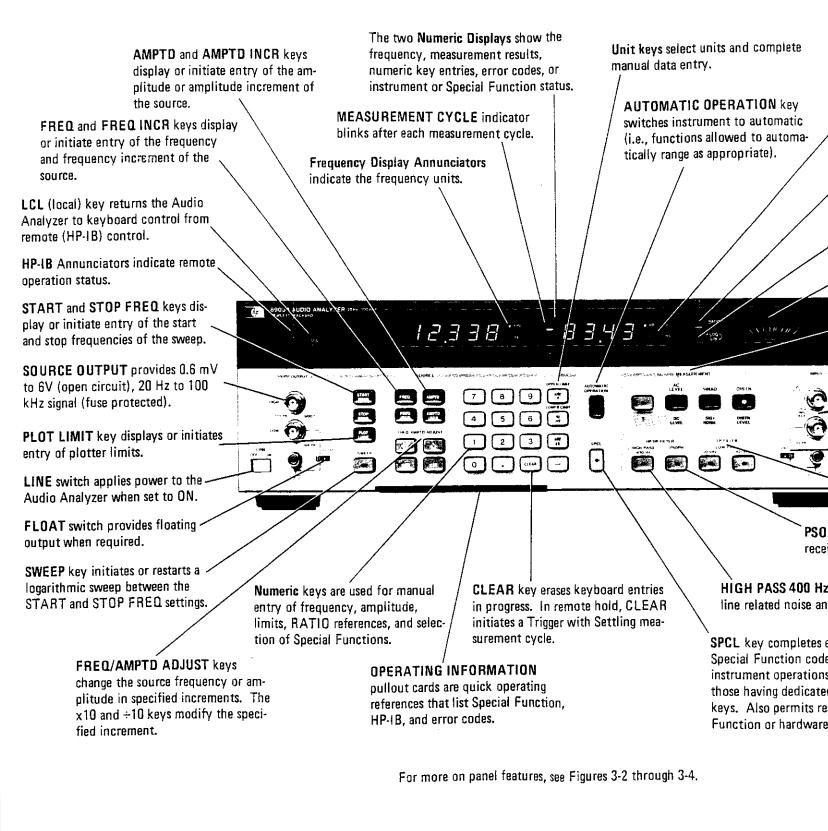
Measurement Display Annunciators indicate the measurement result units.
