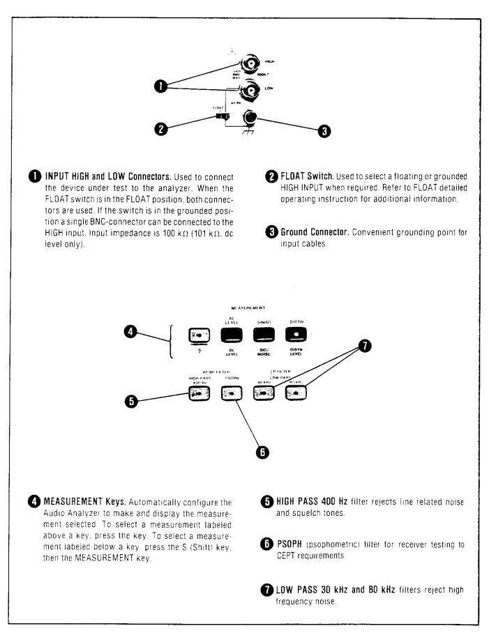
Figure 3-4. Measurement and Input Features
