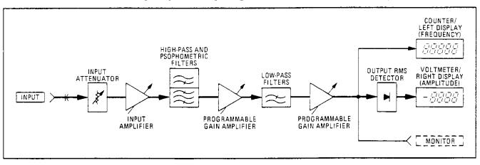
AC Level Measurement Block Diagram
