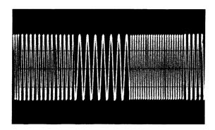
Figure 1-4. Three-Tone Burst Sequence (15 ms Duration)
