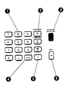
Numeric Keys. Used to enter source frequency and amplitude. incremental values, ratio references. sweep start and stop frequencies, plot limits, and to select Special Functions. Numeric entries are completed by the RATIO, kHz/V (UPPER LIMIT), Hz/mV (LOWER LIMIT), dBV/dB, or SPCL keys. Numeric entries in progress are cleared by the CLEAR key.
