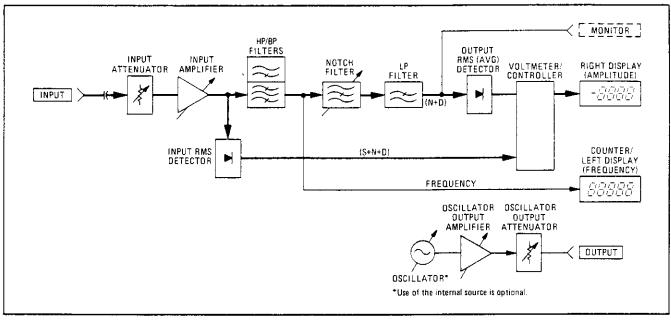
**Distortion Measurement Block Diagram**
