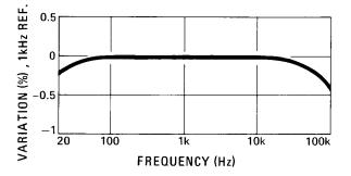
Figure 1-2. Typical Combined Source and AC Level Flatness
