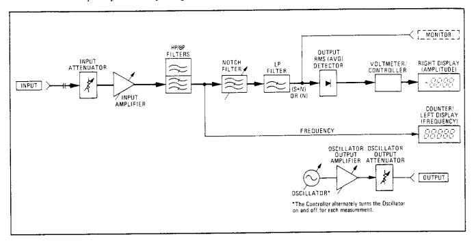
Signal-To-Noise Measurement Block Diagram
