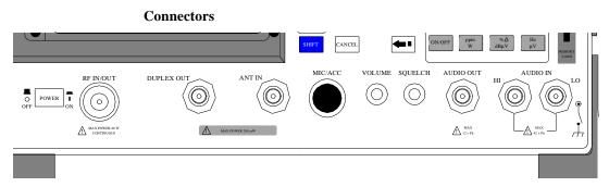
RF IN/OUT Connector – type-N female connector for output signals from the RF Generator, and input signals (60 Watts continuous, or 100 Watts for 10 sec/min) to the RF Analyzer. Nominal impedance is  $50\Omega$ .
