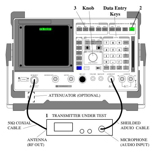
1. Connect the Transmitter as shown.
