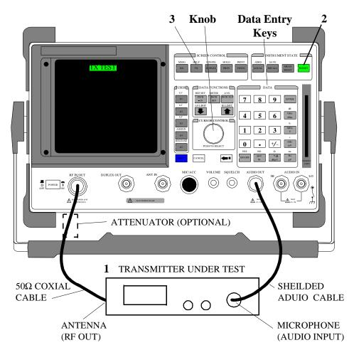
1. Connect the Transmitter as shown.
