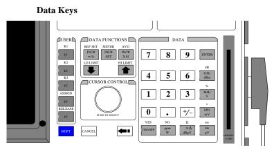
*Data Entry keys*- used to enter or change alphanumeric data (0-9, A-F, ".", "+", or "-") for measurements or field entries. The EEX key is used to enter the exponent for scientific notation.
