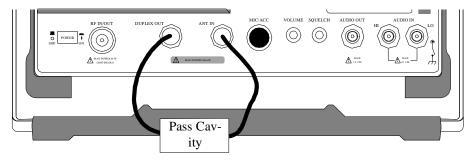
**19.** Adjust the tuning rod to the desired pass frequency.
