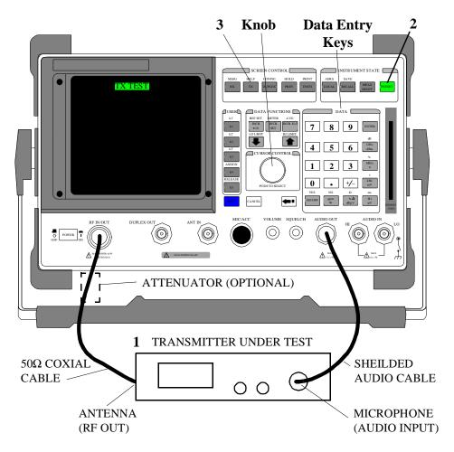
1 Connect the Transmitter as shown.
