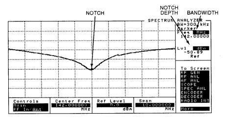
The notch or band-pass frequency can be changed by trimming the coaxial filter in small increments.
