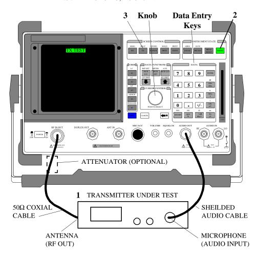
Connect the Transmitter as shown.
