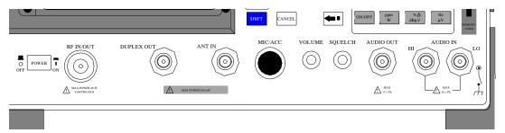
RF IN/OUT Connector – type-N female connector for output signals from the RF Generator, and input signals (60 Watts continuous, or 100 Watts for 10 sec/min) to the RF Analyzer. Nominal impedance is  $50\Omega$ .
