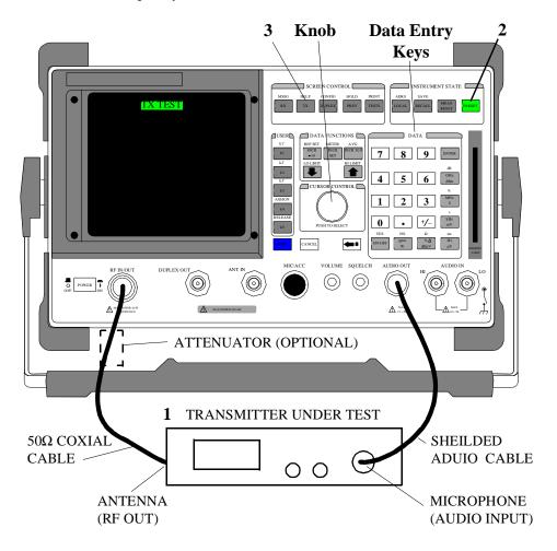
1. Connect the Transmitter as shown.
