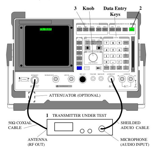
1. Connect the Transmitter as shown.
