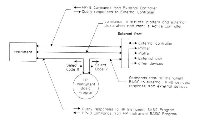
Figure 8-1. HP 89400 Series External and Internal Port
