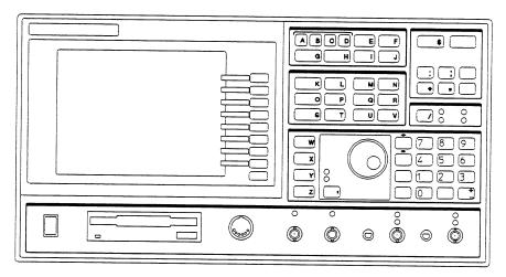
Figure 5-6. HP 89400 series alpha-numeric keys
