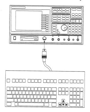
Figure 5-4. Connecting the keyboard.
