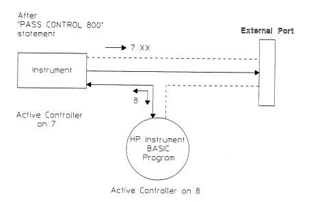
Figure 8-4. Passing Control of the External Interface to the HP 89400-series Analyzer
