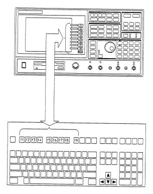
Figure 5-3. Mapping of the HP 89400 Series Softkeys
