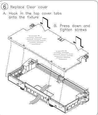
Figure 2-16 (continued). Wiring the HP E1413 Terminal Module
