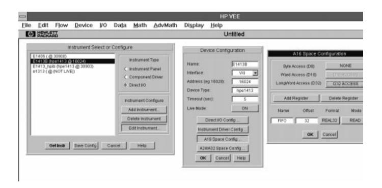
The FIFO register, which is the top of the 64K reading first in first out hardware, is located in A16 address space at offset 32. Each time this register is read, one reading is removed from the hardware FIFO.
