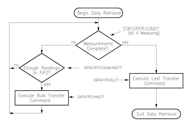
Figure 4-3. Fastest Reading Transfer
