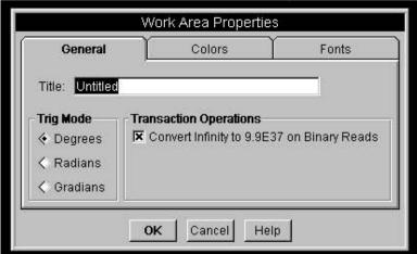
This sets up HP VEE so it can directly access data from the HP E1313/E1413 FIFO and CVT registers. This is required because the HP E1313/E1413 has implemented IEEE 754 Floating Point Format which includes special codes for "plus infinity", "minus infinity", and "not a number". These special codes causes a floating point math error in HP VEE, thus they must be converted to a number which HP VEE can handle such as 9.9E37.
