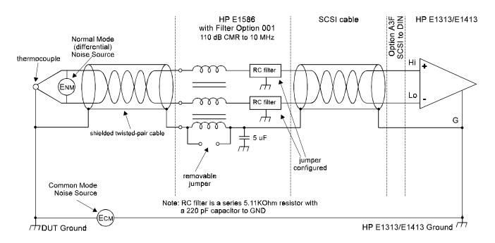
Figure F-1. HF Common Mode Filters
