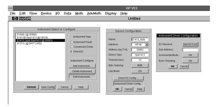
The HP E1406A Command Module should be set so that all of its memory is available. The RAM switches should be set for 2M RAM, 0 Shared. Then the following portion of an HP VEE program configures this memory as Nram. You need to use this procedure because the exact size and address may change based on how an HP E1406A is configured.
