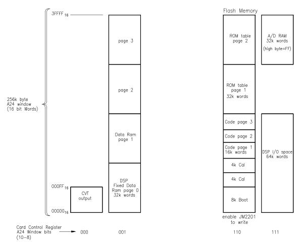
Figure D-2 A24 Memory Mapping
