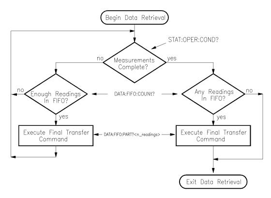
Figure 4-2. Controlling Reading Count
