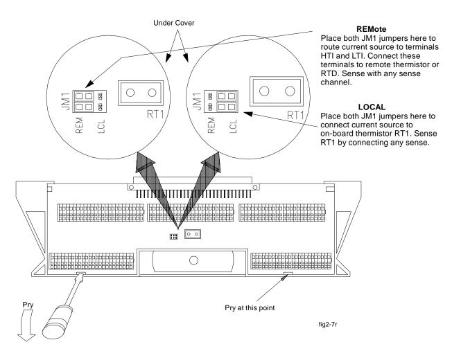
Figure 2-11. Temperature Sensing for HP E1313 Terminal Module
