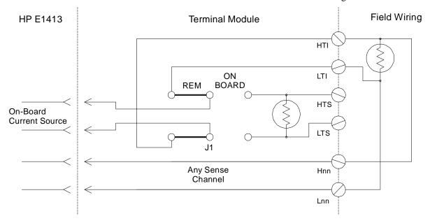
Figure 2-6. Remote Thermistor or RTD Connections
