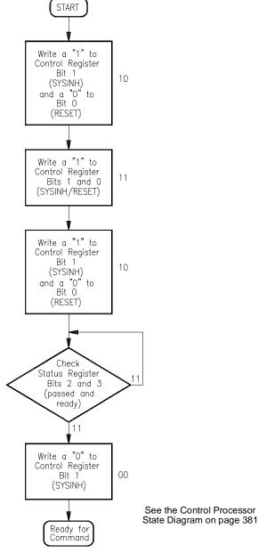
Figure D-3. Resetting the HP E1313/E1413
