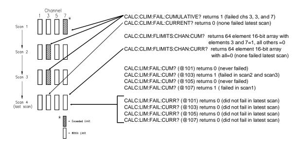
Figure 4-8. Querying Limit Test Results
