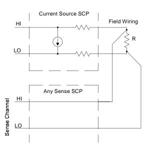
Figure 3-2. Resistance Measurement Sensing
