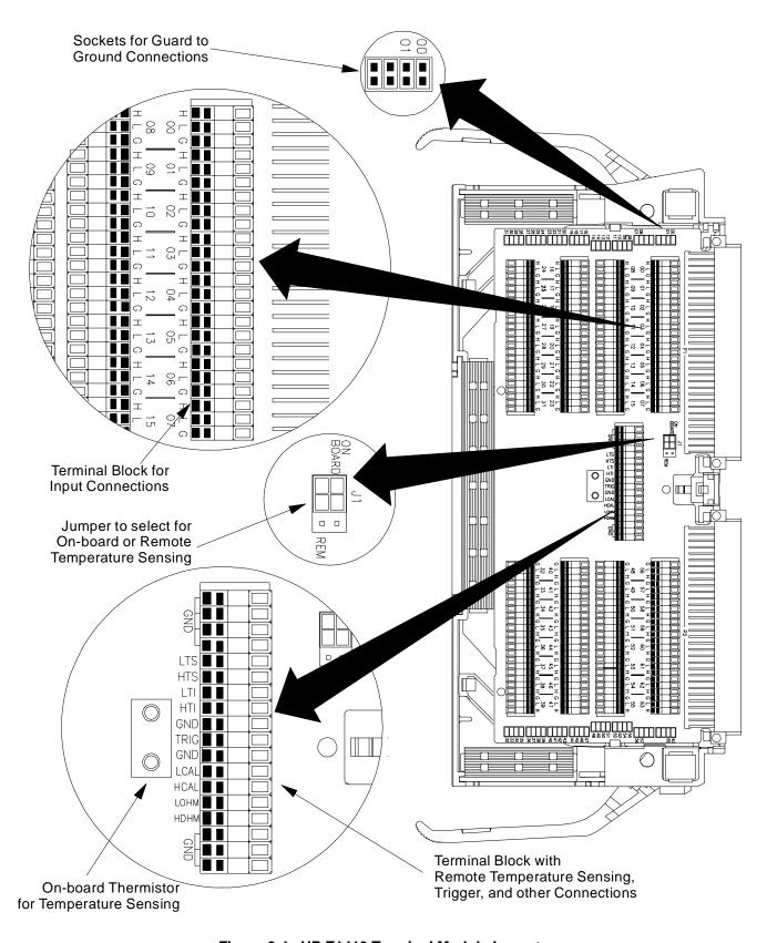
Figure 2-4. HP E1413 Terminal Module Layout
