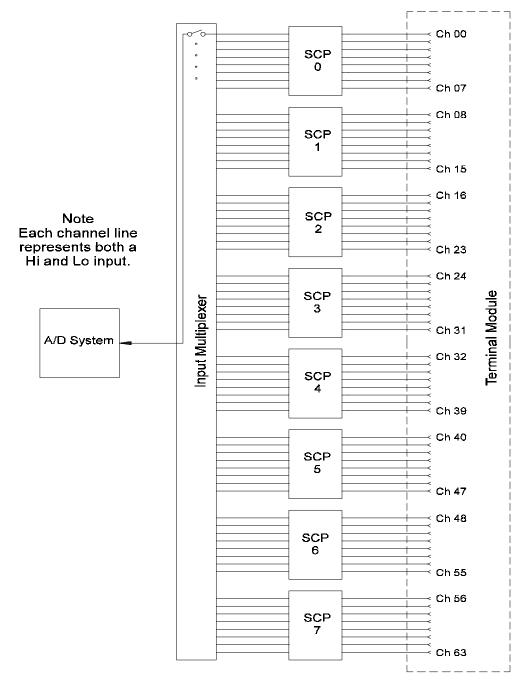
Figure 2-1. Channel Numbers at SCP Positions
