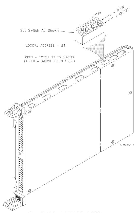
Figure 1-2. Setting the HP E1413 Logical Address
