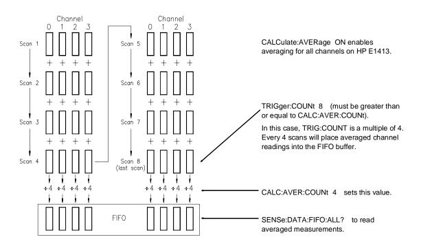
Figure 4-7. Averaging Channel Measurements
