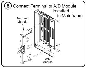
Figure 2-15. Wiring and Connecting the HP E1313 Terminal Module
