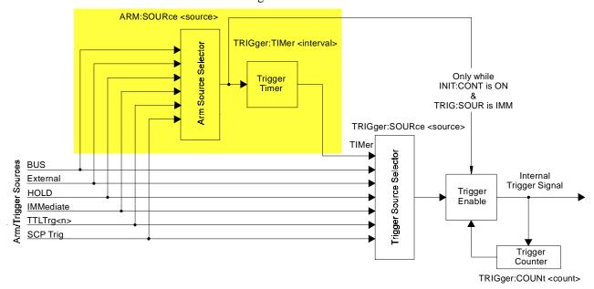
Figure 3-4. Logical Arm and Trigger Model
