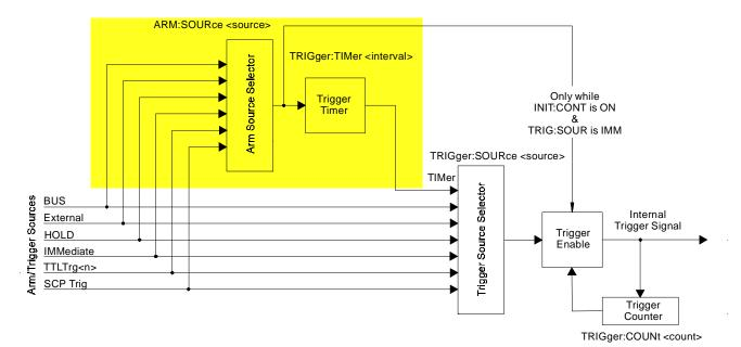
Figure 5-1. Logical Trigger Model
