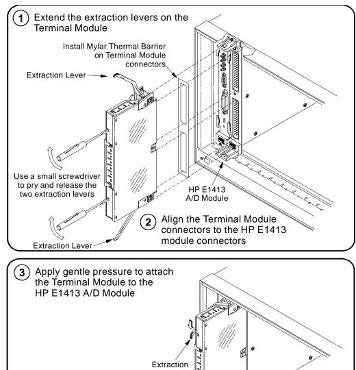
Push in the extraction levers to lock the Terminal Module onto the HP E1413 A/D Module
