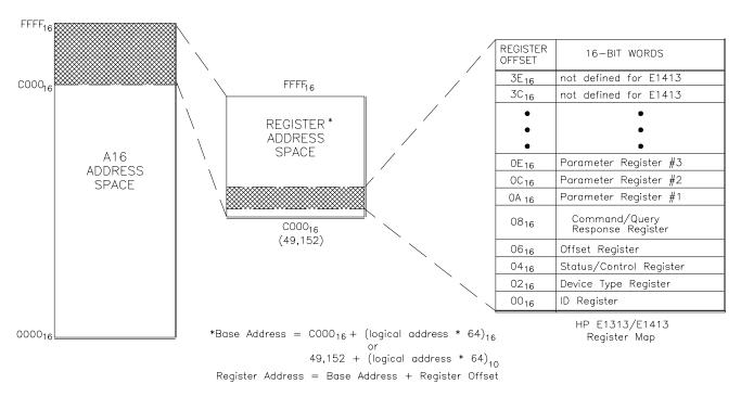
Figure D-1. HP E1313/E1413 Registers within A16 Address Space
