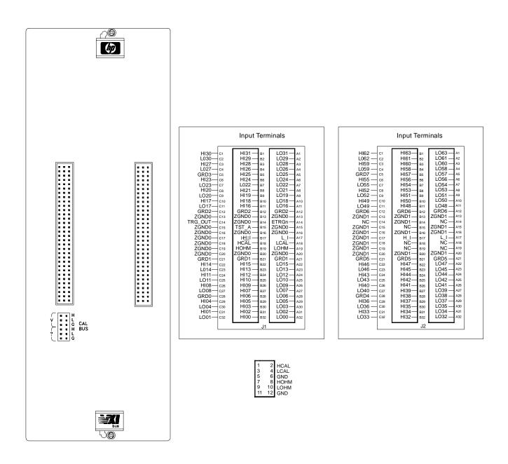
Figure 2-26. HP E1313 Connector Pin-Signal List
