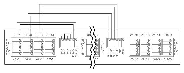
One HP E1586 Terminal Panel Measuring Three Thermistors on Reference Channels 100, 101, 102
