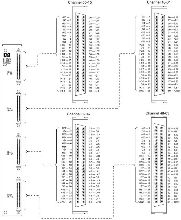
Figure 2-24. HP E1413 Option A3F Pin-out
