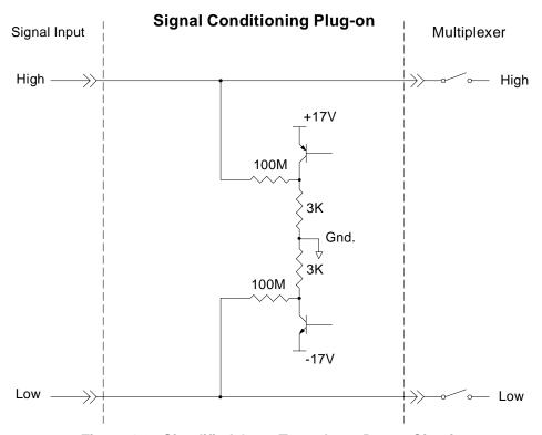
Figure 4-9. Simplified Open Transducer Detect Circuit
