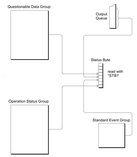
Figure 4-5. Simplified Status System Diagram
