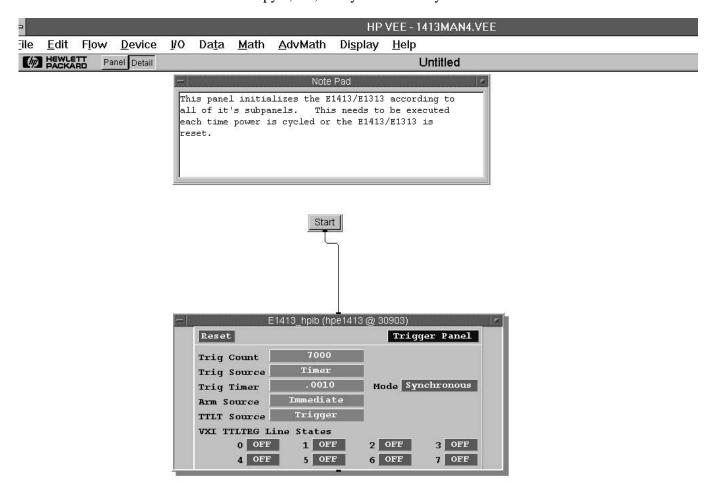
This part of the program starts the measurement and then transfers the readings to the computer. The READ BINARY x BYTE ARRAY:9 reads the IEEE 488.2 arbitrary block header. The block header has the form of #ndd where:
