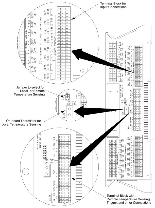
Figure 2-3. HP E1313 Terminal Module Layout
