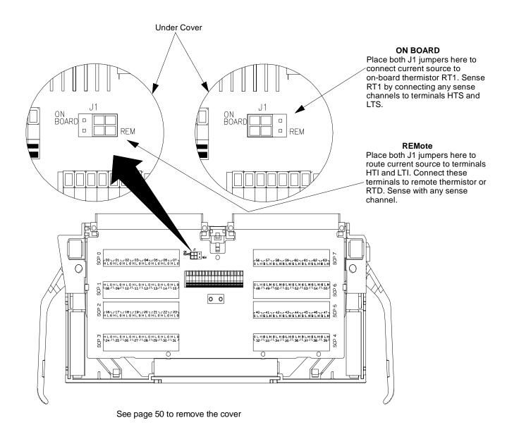
Figure 2-12. Temperature Sensing for HP E1413 Terminal Module
