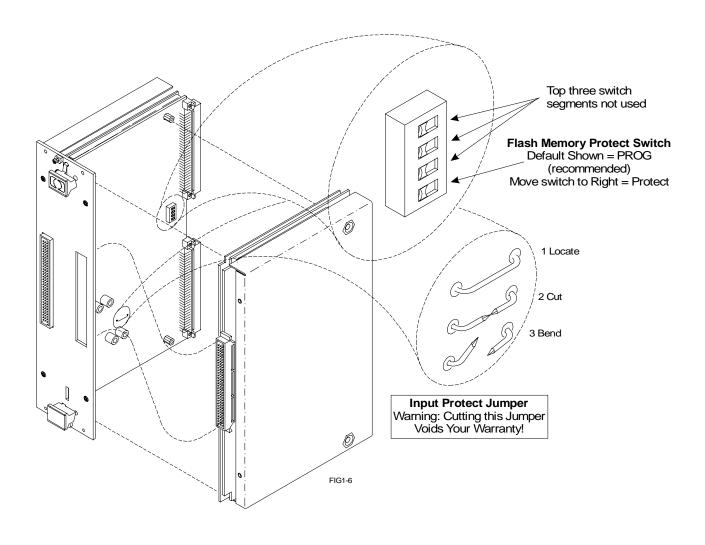
Figure 1-3. Locate and Access JM2201 and JM2202 on HP E1313
