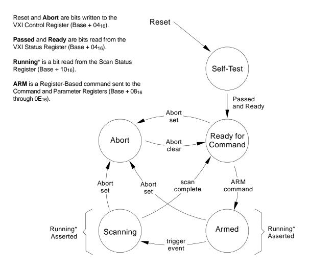
Figure D-7. Control Processor State Diagram
