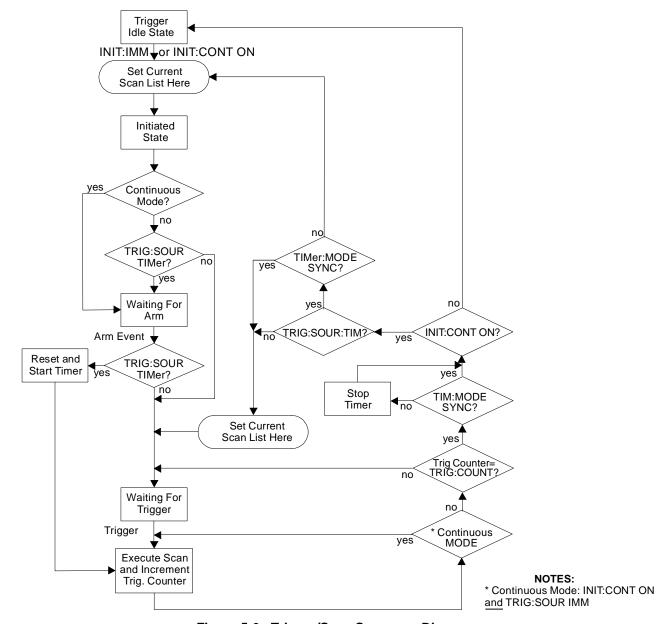
**Event Sequence** Figure 5-6 shows how the module responds to various trigger/arm configurations.
