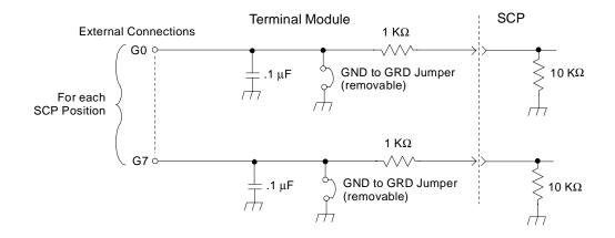
Figure 2-9. GRD/GND Circuitry on Terminal Module
