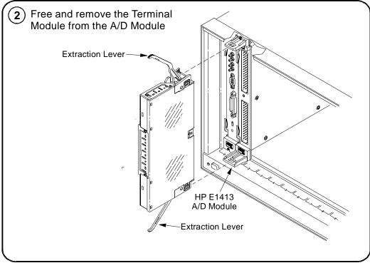
Figure 2-18. Removing the HP E1413 Terminal Module
