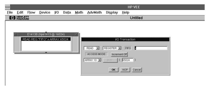
This sets HP VEE up to read the register that in step 2 we named "FIFO" and store the results in variable X.
