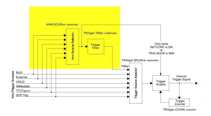
Figure 5-5. Logical Trigger Model
