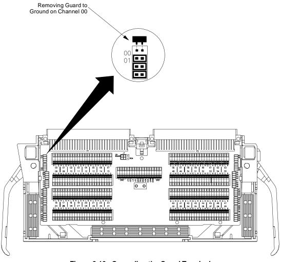
Figure 2-10. Grounding the Guard Terminal
