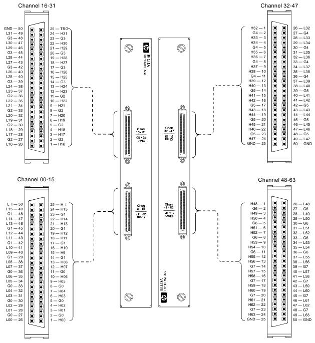
Figure 2-23. HP E1313 Option A3F Pin-out
