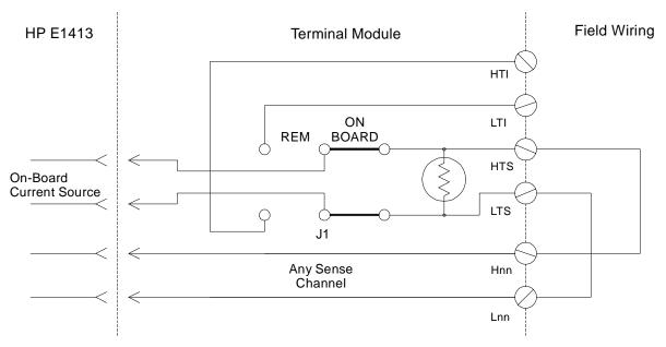
Figure 2-7. On-Board Thermistor Connections
