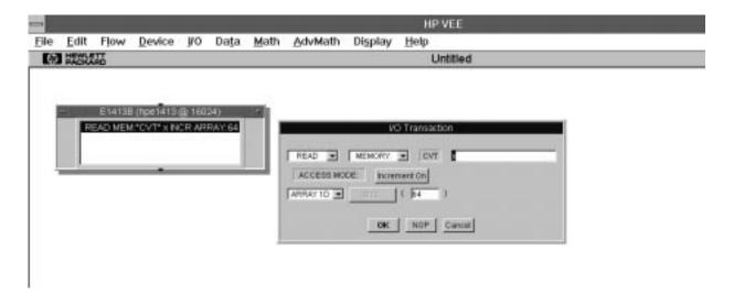
This sets up HP VEE to read the CVT Current Value Memory that in step 2 we named "CVT" and store the results in variable X.
