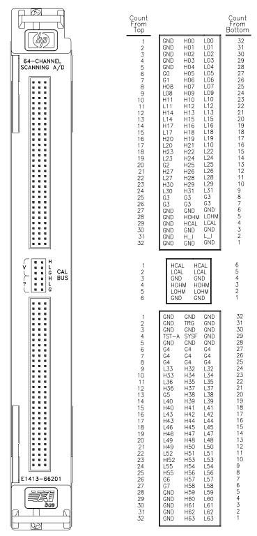
Figure 2-27. HP E1413 Connector Pin-Signal List
