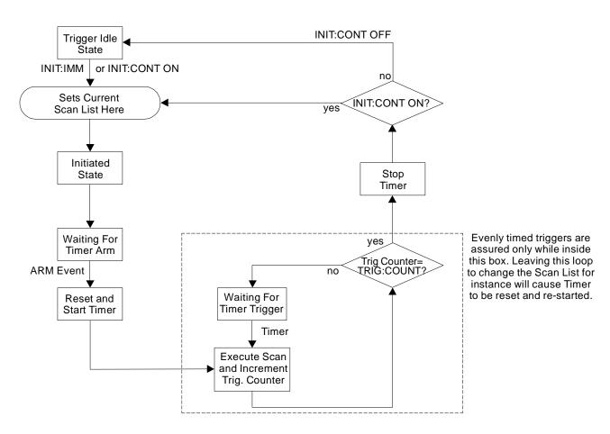
Figure 5-7. Asynchronous Mode Sequence
