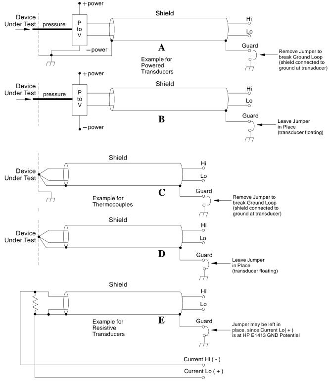
Figure 2-8. Preferred Signal Connections
