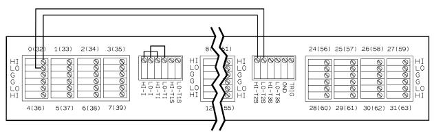
One HP E1586 Terminal Panel Measuring One Thermistor on Reference Channel 100
