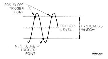
Figure 4-18. Positive and Negative Trigger Points
