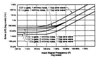
Graph 1. Frequency Resolution Error: Noise on the input signal and internal uncertainties affects Frequency and Period measurements. For Period, invert the period (P) of the input
