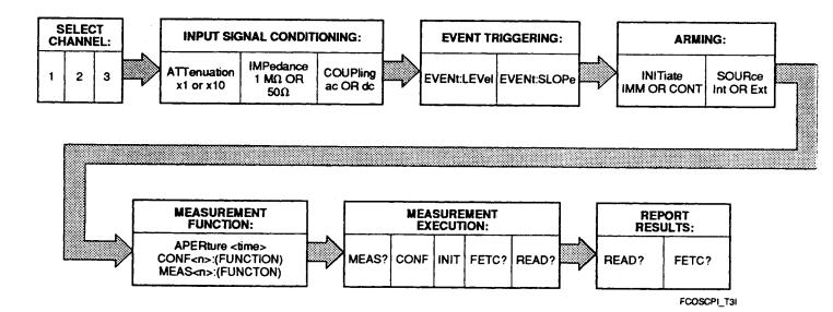
Figure 4-1. Overall SCPI Measurement Flow
