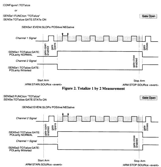
Figure 3. Totalize 2 by 1 Measurement
