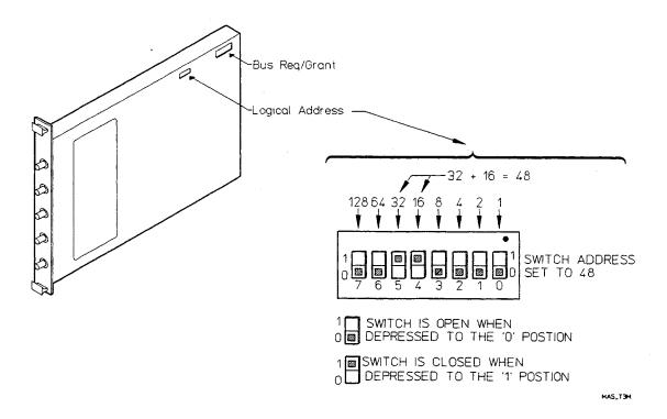
Figure 2-2. HP E1420B Address Switch Location and Selection
