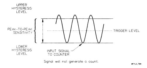
Figure 4-13. Trigger Level Set Below Midpoint of Input Signal
