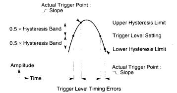
The following equations define the general interpretation of its component error terms for a measurement. These equations should be summed together to obtain the overall Trigger Level Timing Error.
