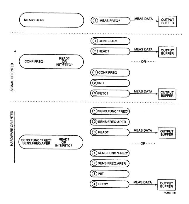
Figure 4-2. SCPI Measurement Capability
