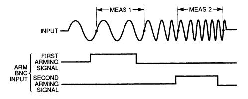
Figure 4-21. Use of External Arming to Measure Frequency
