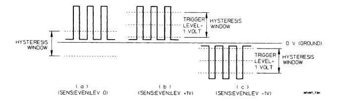
Figure 4-17. Hysteresis Window and Trigger Level
