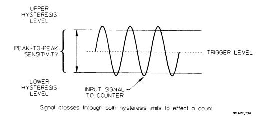
Figure 4-11. Acceptable Peak-to-Peak Amplitude
