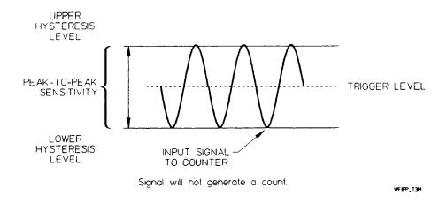
Figure 4-12. Insufficient Peak-to-Peak Amplitude
