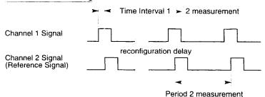
Figure F-1. Phase Measurement Definition and Timing
