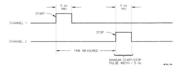
Figure 4-6. Time Interval Measurement
