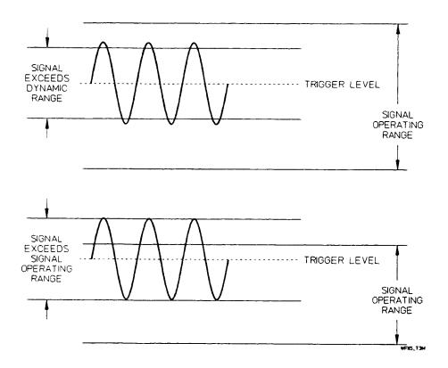
Figure 4-9. Invalid Input Signal Conditions
