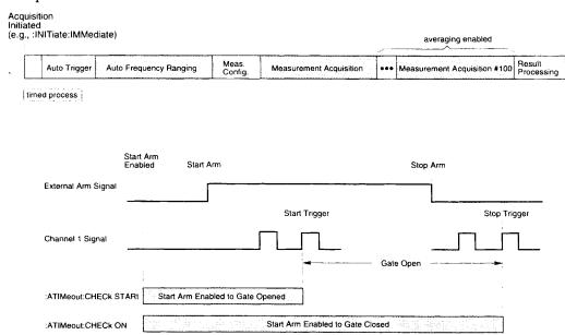
Figure F-2. Acquisition Timeout Timing Example
