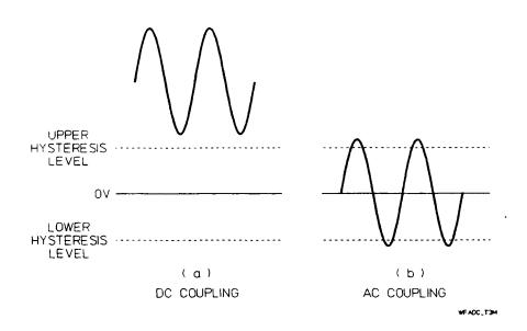
Figure 4-15. Ac-Dc Coupling
