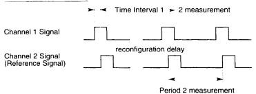
Figure F-1. Phase Measurement Definition and Timing
