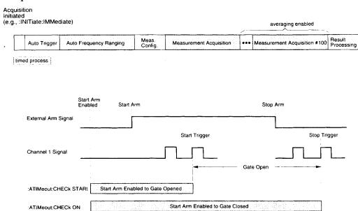
Figure F-2. Acquisition Timeout Timing Example
