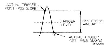
Figure 4-16. Trigger Level and Actual Trigger Point
