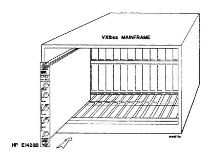
Figure 1-2. HP E1420B Mainframe Installation
