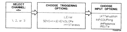
Figure 4-8. SCPI Signal Conditioning Flow
