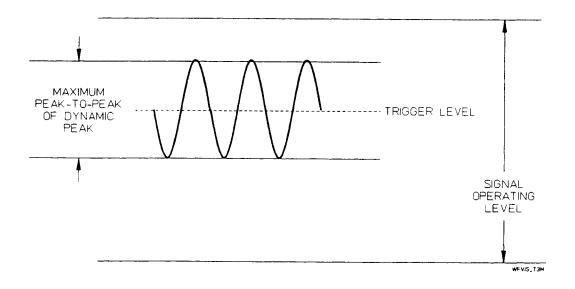
Figure 4-10. Valid Input Signal Conditions
