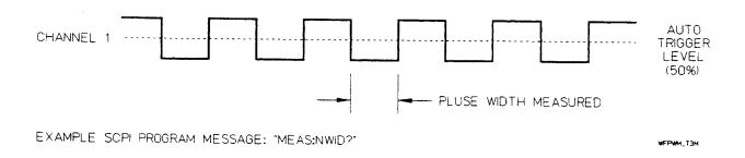
Figure 4-4. Pulse Width Measurement
