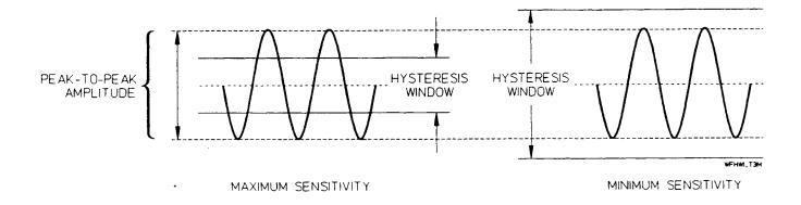
Figure 4-14. Hysteresis Window and Input Sensitivity
