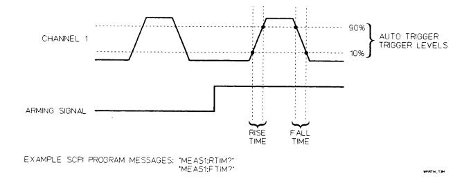
Figure 4-5. Rise | Fall Time Measurements
