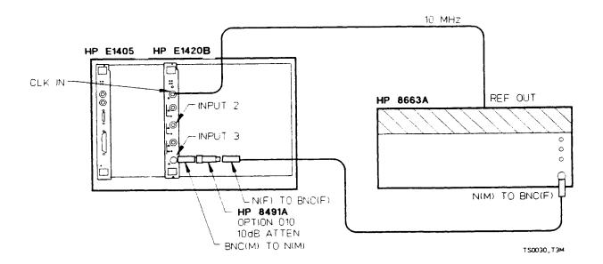
Figure C2. Option 030 Test Setup
