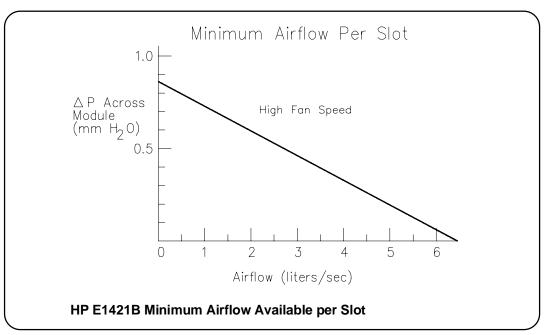
Fan set to "Variable": Quiet operation (approx. 75% airflow) at <30 °C ambient temperature and high speed operation at >40 °C ambient temperature.
