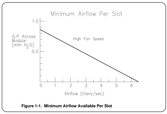
The mainframe has a fan chamber with one circulation fan. The speed of the fans is controlled by the ambient temperature of the air drawn into the mainframe. Air from the fan chamber is forced through the right side of the plug-in modules. The air passes through the installed modules and escapes out the left side of the mainframe.
