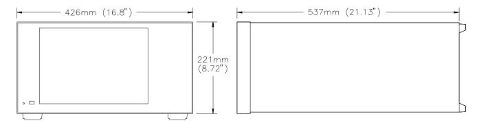
**Mainframe Weight** HP E1421B: 15.0 Kg (33.0 lbs) with no modules installed.
