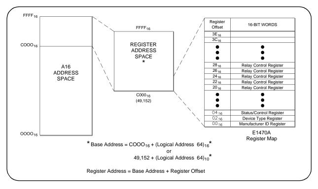
Figure B-1. Register Address Locations Within VXI A16
