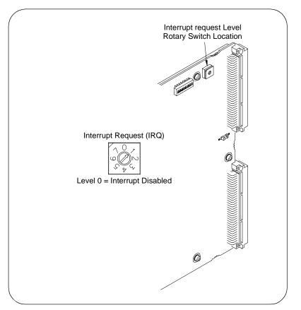
Figure 1-5. Setting the Interrupt Request Level Switch
