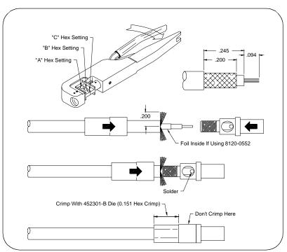
Figure 1-7. Assembling SMB Jacks and Cables
