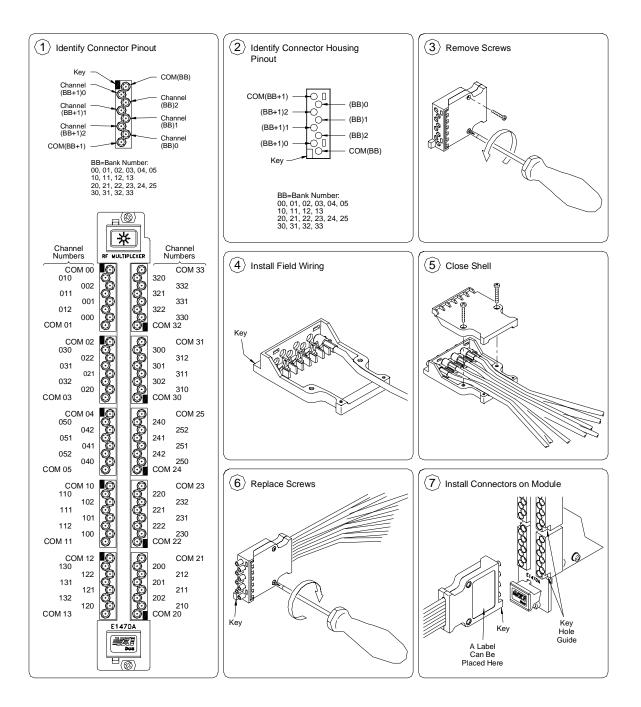
Figure 1-6. Installing User Wiring
