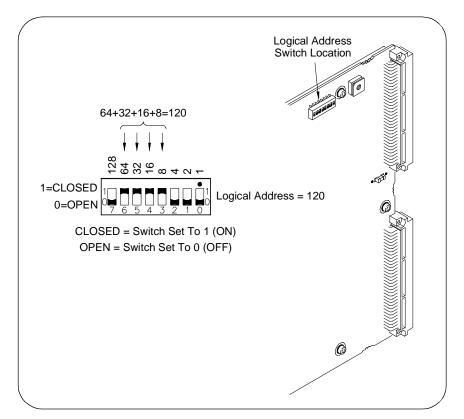
Figure 1-4. Setting the Logical Address Switch
