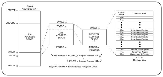
Figure B-2. A16 Address Space in the E1406 Command Module
