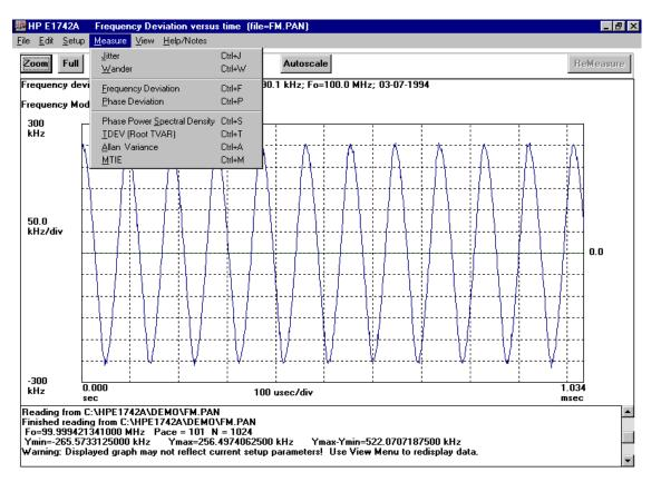
**MEASURE MENU VS VIEW MENU**. The choices on these two menus are very similar, however the action performed by the instrument is quite different. Selecting any of the choices on the **Measure** menu will cause the instrument to initiate a measurement and acquire a new set of data points and perform the selected result processing. Selecting any of the choices on the **View** menu will cause the instrument to perform the selected calculations *on the currently acquired data*.
