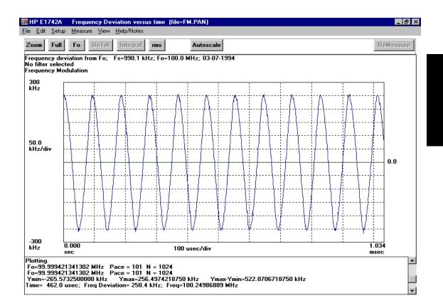
The last line of the display shows the x value of the cursor (time), the difference between the measured frequency and the carrier frequency Fo (Freq Deviation), and the absolute frequency value (Freq).
