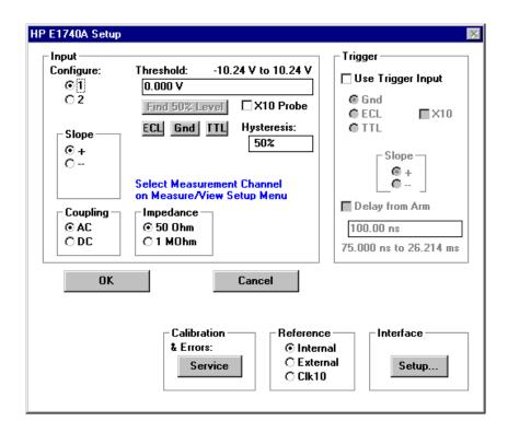
This is the **HP E1740A Setup** menu to configure the instrument to measure the BPSK signal.
