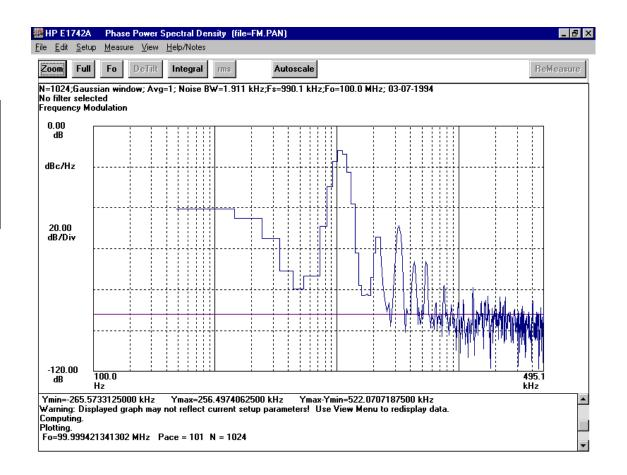
This display was computed from the "fm.pan" data. This is the power spectral density plot of the modulating tone. The 11 kHz modulation is easily seen on this display, as well as other modulation products.
