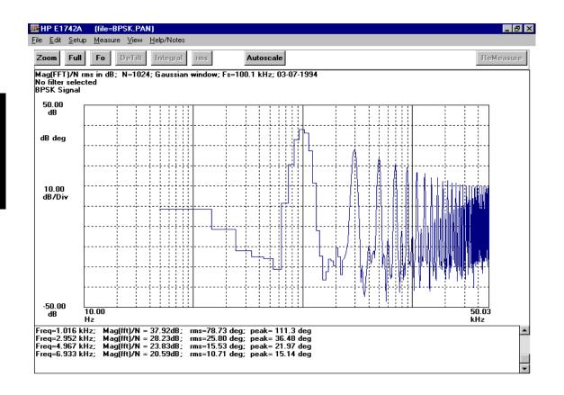
Using the cursor and clicking on each peak in the spectrum, the characteristic odd harmonics of the square wave phase modulation can be seen. Note that this is not the same view as a spectrum analyzer would display (spectrum of the modulated carrier), but a direct view of the spectral content of the modulation.
