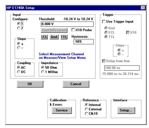
This window is used to specify the measurement hardware configuration. The window is divided into five or six separate areas. **Input Configure**, **Trigger, Calibration & Errors, Reference**, and **Interface** are common to all HP E174XA products. You will only need to modify the **Input Configure** and **Trigger** selections for most measurements. In most cases, changes become effective when you click the OK button and close this dialog box.
